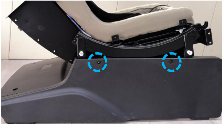
A、remove the 2 screws
