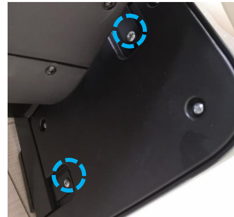
D、remove the 2 screws at front end
