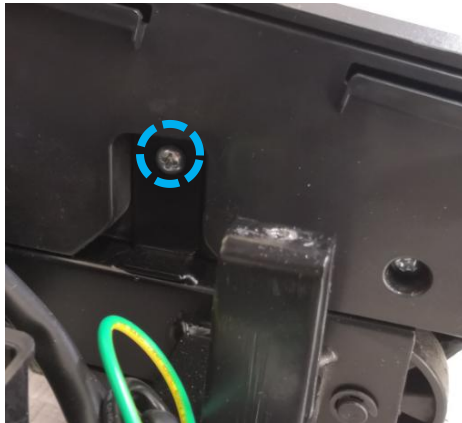
C、remove the screw at rear end
