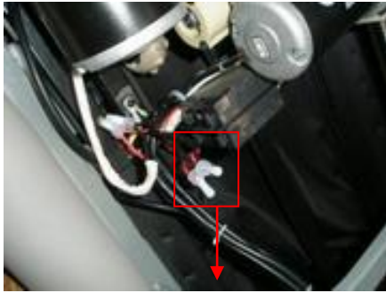
Close-end wire connector of tapping motor
