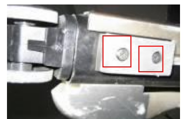
Screws securing the rubber support
