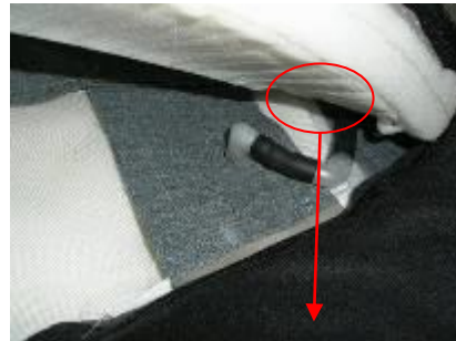
Pull out the hoses
