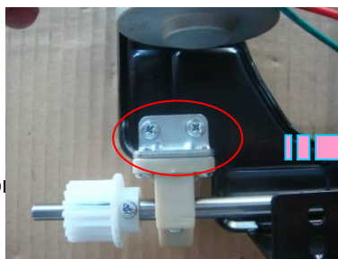
Screws (5pcs) securing the Rolling motor
