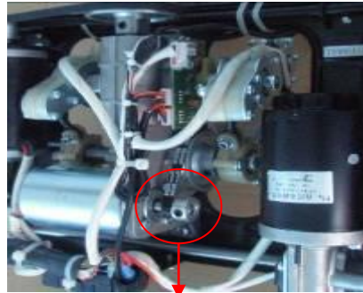
Screws securing the tapping motor
