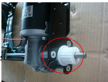
Screws (5pcs) securing the Rolling motor
