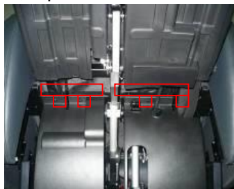
Screws(12pcs) securing the front panel
