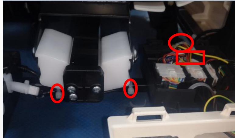
B.cut cable tie, disconnect the terminal
