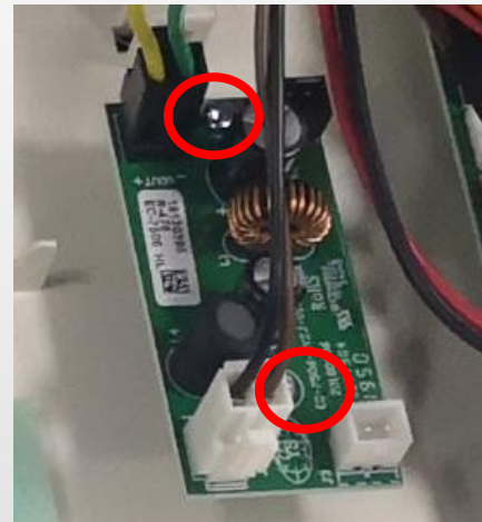
disconnect the terminals, remove 5 screws
