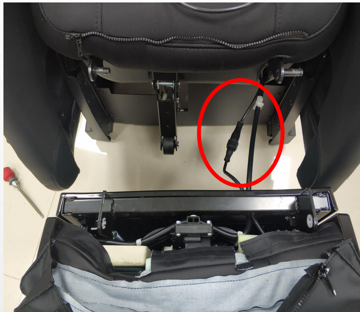
B. disconnect the terminal and air hose
