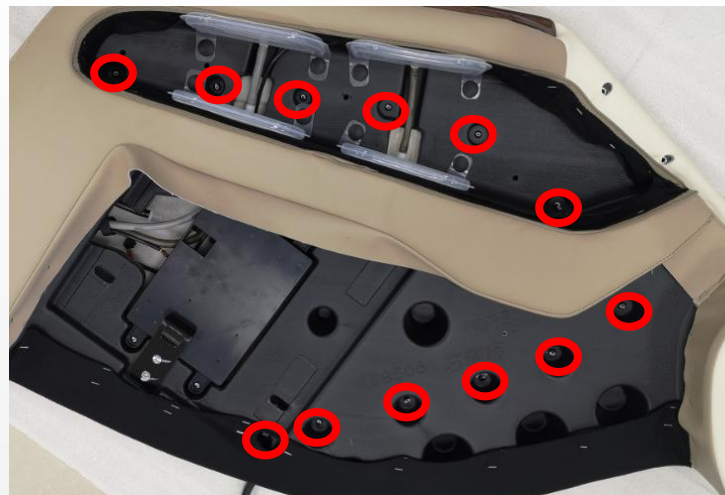
M .remove the screws
