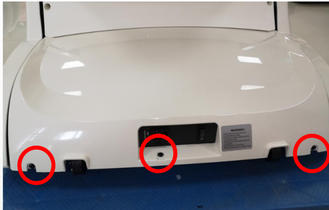
A.remove 3 screws, open themain PCB box
