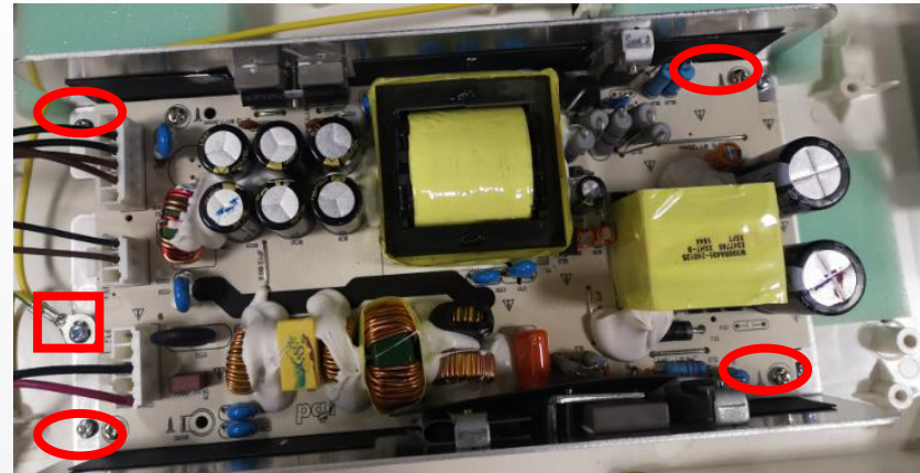
disconnect the terminals, remove 5 screws
