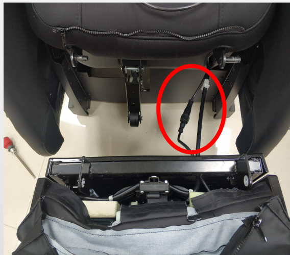
C. disconnect the terminal and air hose
