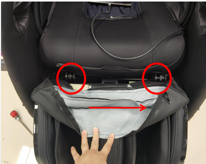
A. Remove the blocking on both sides of the legrest
