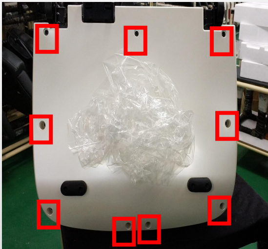
D. remove 9 screws
