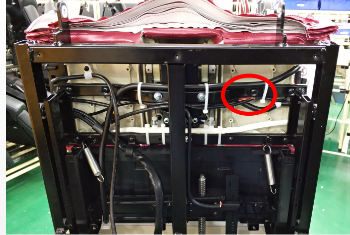
B. Cut off button, Unplug all terminals
