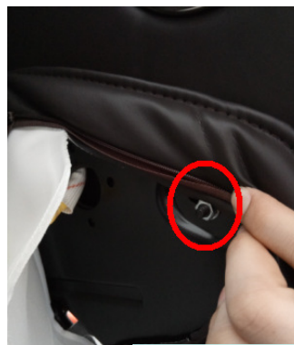
拆除固定肩部的螺母 Loose and screw the nut
