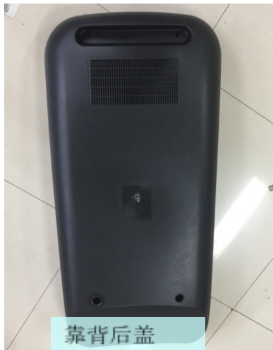
取下固定靠背后盖的4枚螺丝 Slack and remove 4 screws fixing the cover
