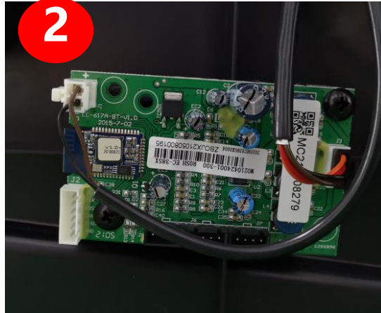
disconnected the terminals and remove 4 screws
