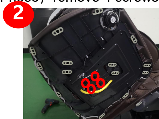
disconnected the terminal and air hose, remove 4 screws
