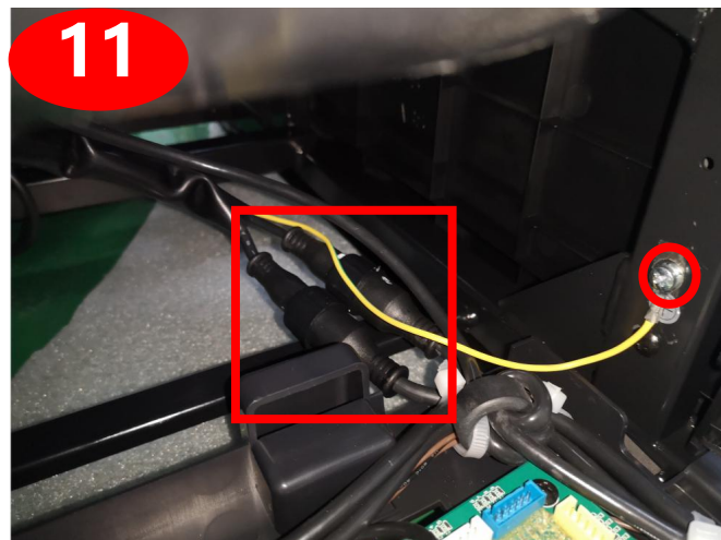
disconnected the terminals, remove the screw
