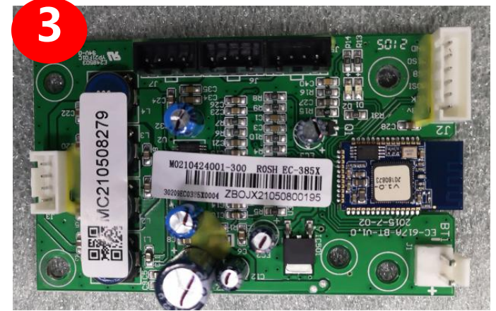
remove the Bluetooth PCB
