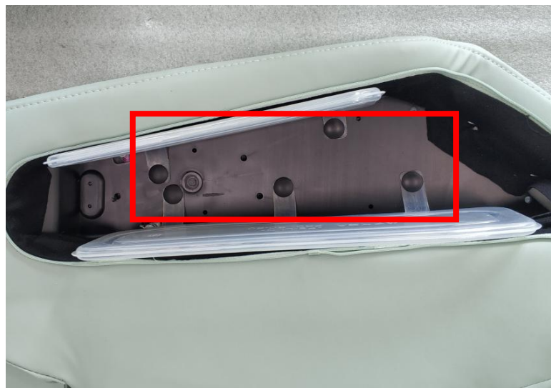
remove the screws
