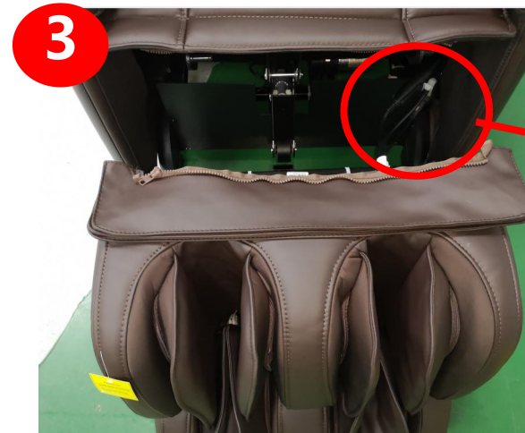
disconnected the terminal and air hose
