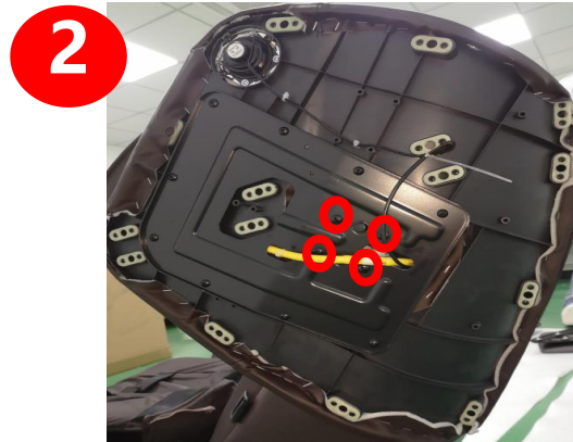
disconnected the terminal and air hose, remove 4 screws
