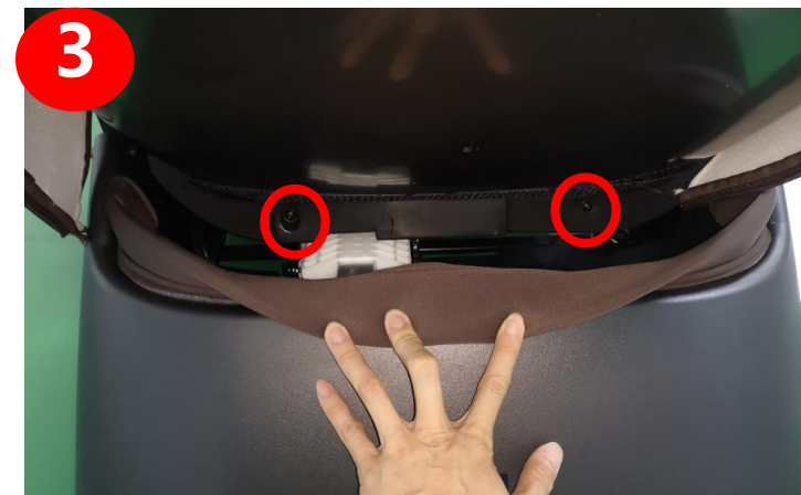
remove 2 screws on the bottom
