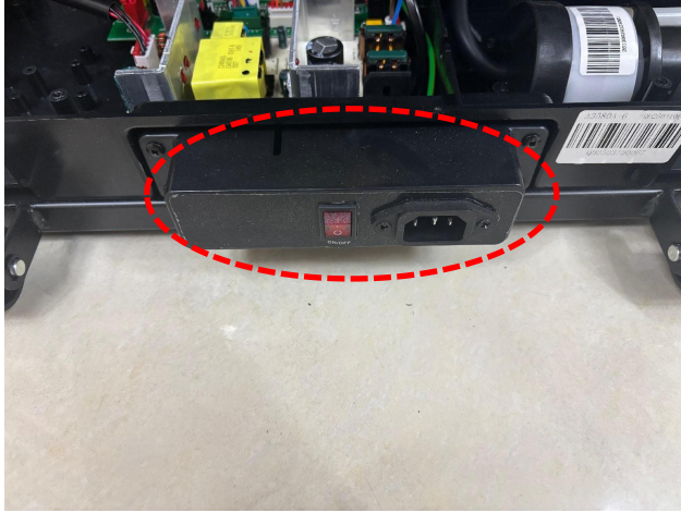
power switch box assembly
