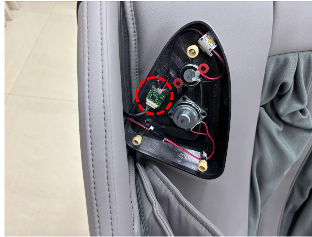
Voice control board
