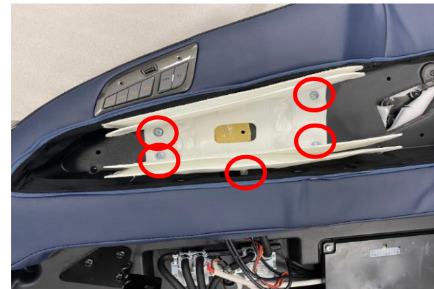
remove 4 screws and remove air bag
