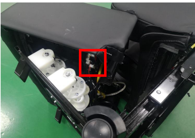
i.remove 2 screws, cut cable tie
