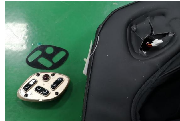
disconnected the terminal and remove the control
