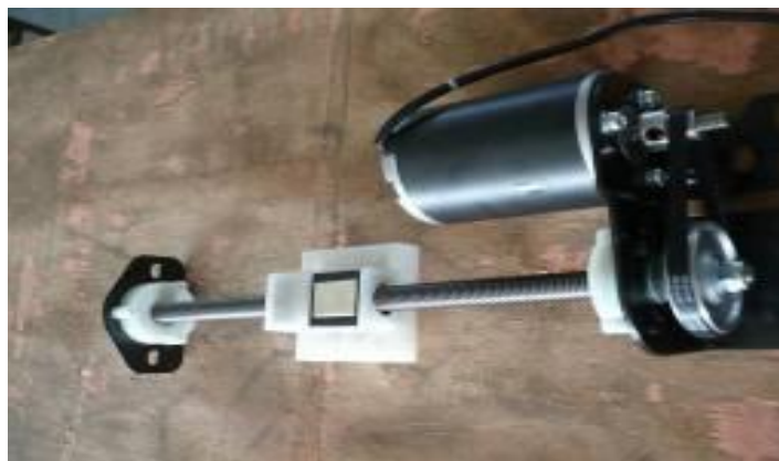
Calf telescopic motor assembly
