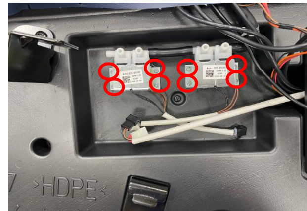
remove 8 screws, remove air valves
