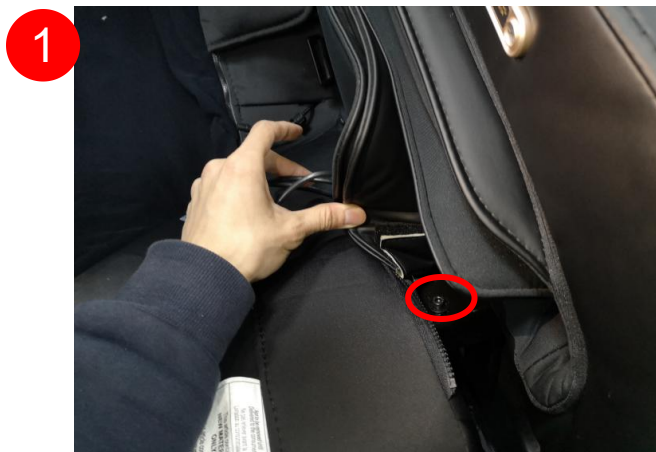
remove the screw of right side panel
