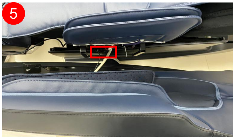
cut cable, discontent terminal and air hose
