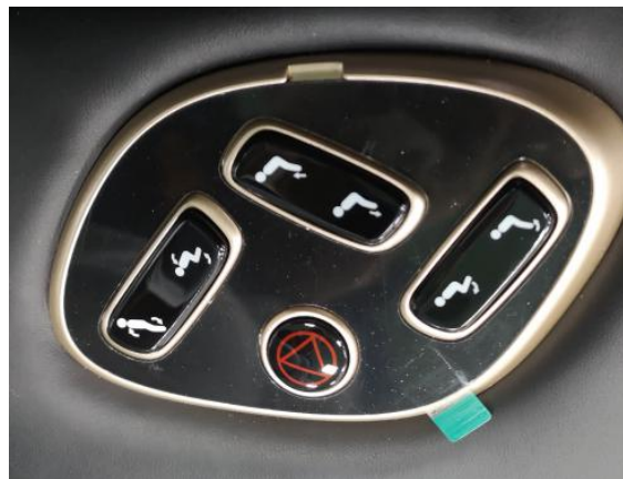
Pry off the key board assembly along the edge
