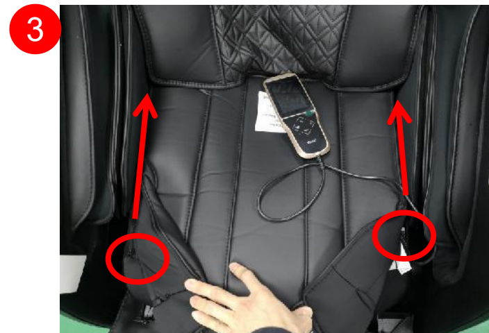
cut cable tie, reemoveheat shrinkable sleeve
