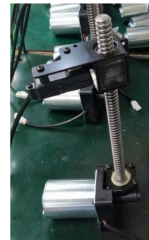
remove leg telescopic motor assembly
