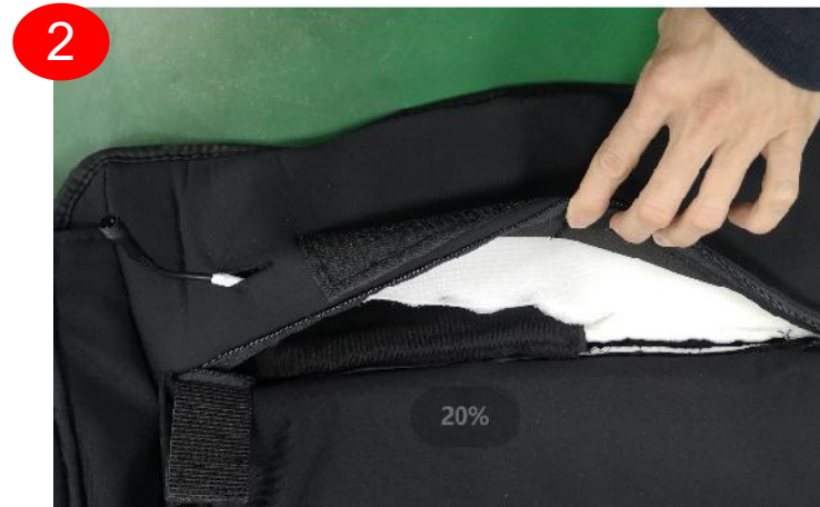
disconnect terminals, remove heater
