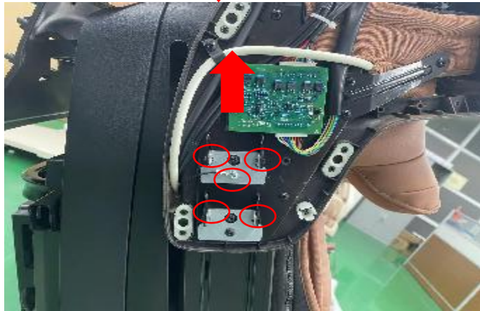
M .remove 5 screws, Extract the right shoulder assembly upwards
