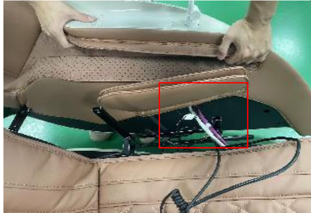
B. discontent the terminal and air hose
