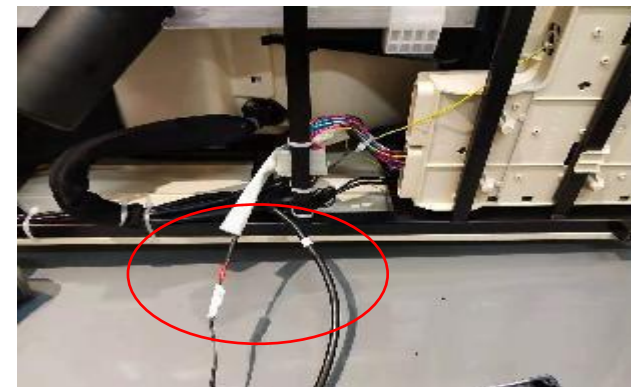
C.disconnect the air hose and terminal
