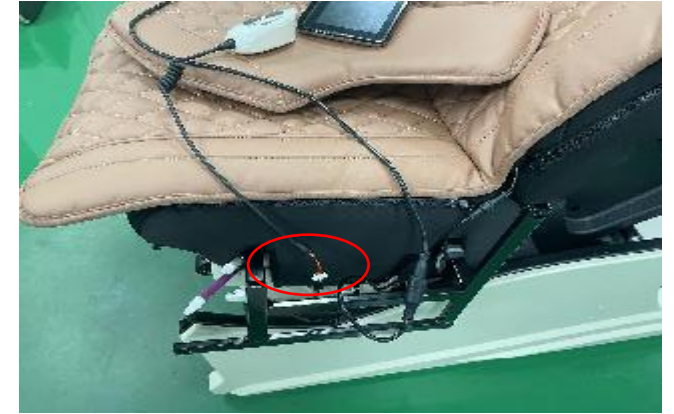
C. disconnected the terminal
