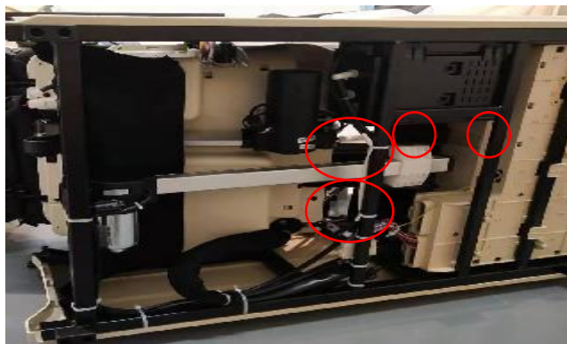
B.cut cable tie, remove 2 screws
