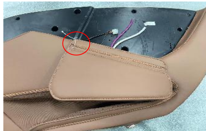
B. separate the leather from plastic screw
