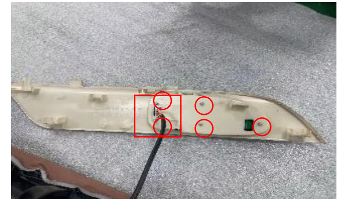
F. remove 5 screws, discontent the tterminal
