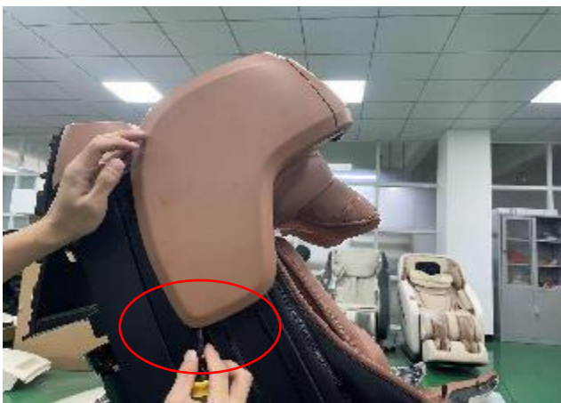
J .open the cover with a “—” screwdriver
