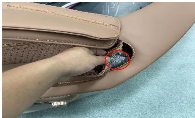
B. separate the leather from plastic screw
