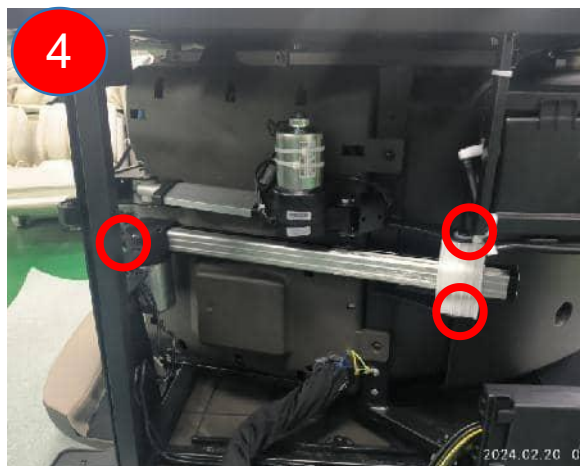
Remove the front pin and rear screw
