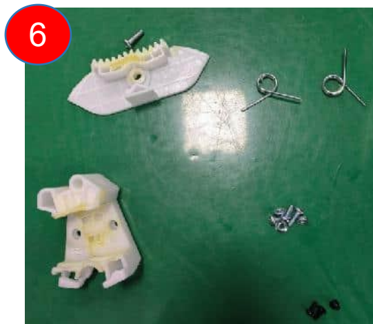
Remove the guide rail adapter plate
