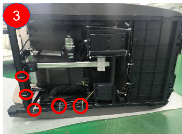
cut the cable tie
