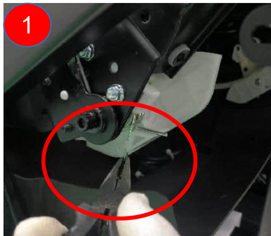
clamp the spring open with apointed nose pliers
