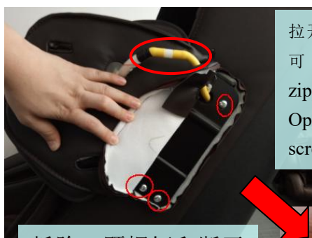
拆除 3 颗螺钉和断开 气管 Demolition of 3 screws and Disconnect air hose terminal
