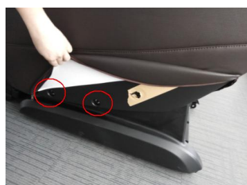
拆除 2 颗螺钉 Demolition of two screws
