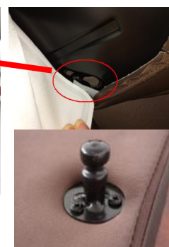
将侧板向前推动至销轴移出 卡槽 Remove the side panel push forward to pin card slots
