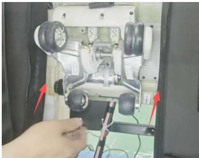
14. Move the movement gears and take out the movement at the gap
