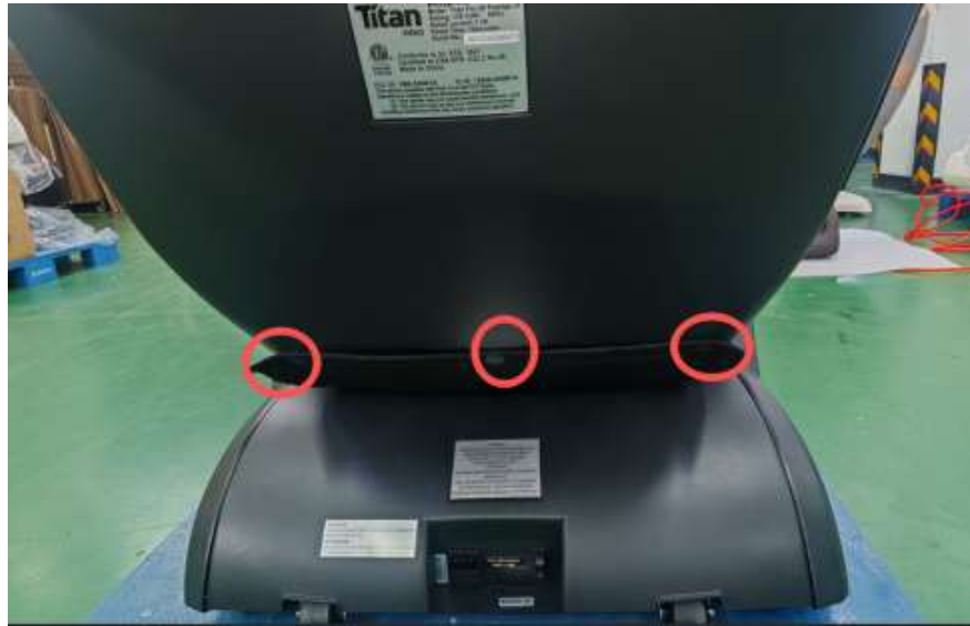
2.Pull out the cloth sleeve pin and remove the rear cover
