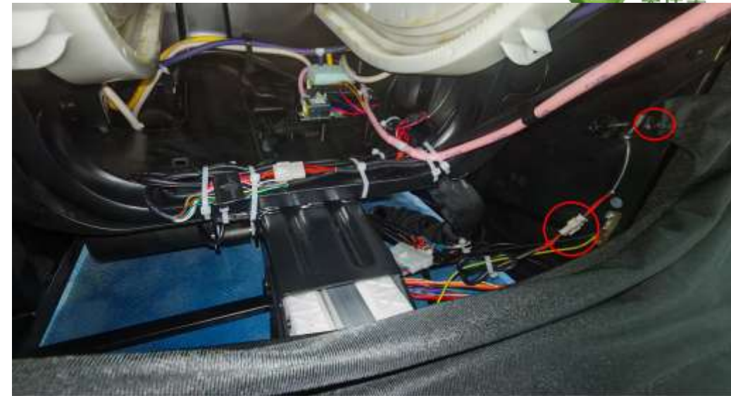
3.Remove 1 screw and disconnect the terminal
