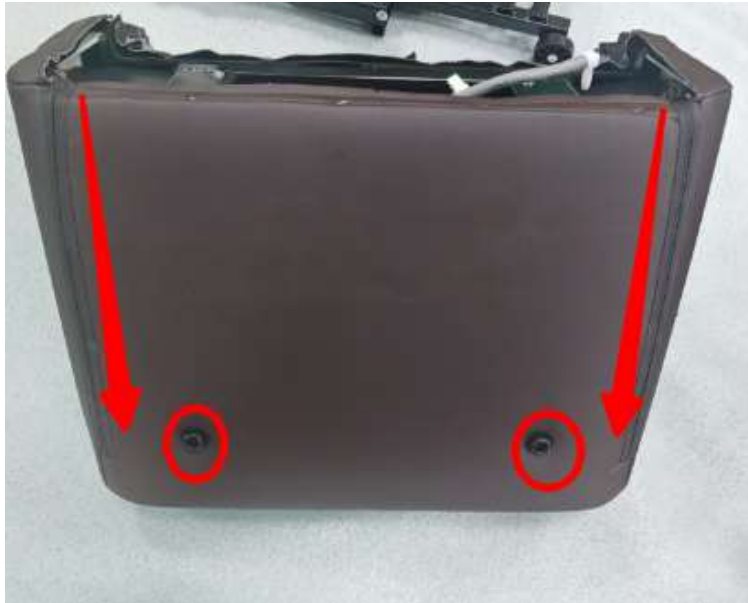
10. Remove 2 screws and unzip
