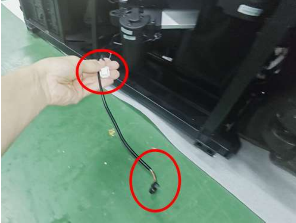
7.Disconnect the terminal of the leg lift push rod
