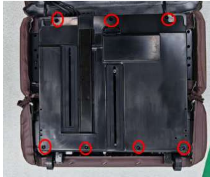
2. Remove 7 screws and remove the cover plate
