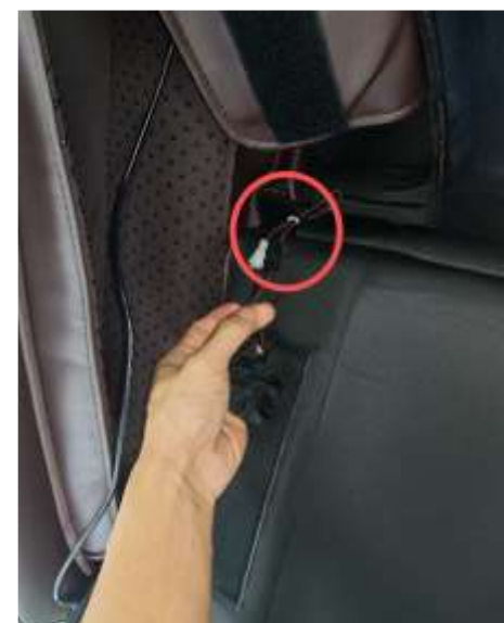
6.disconnecting the terminals
