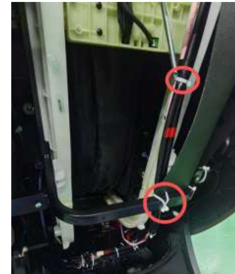
7.Cut off the tie
