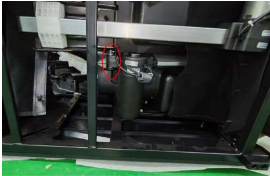
4.Pull off the cotter pin and remove the lower pin shaft
