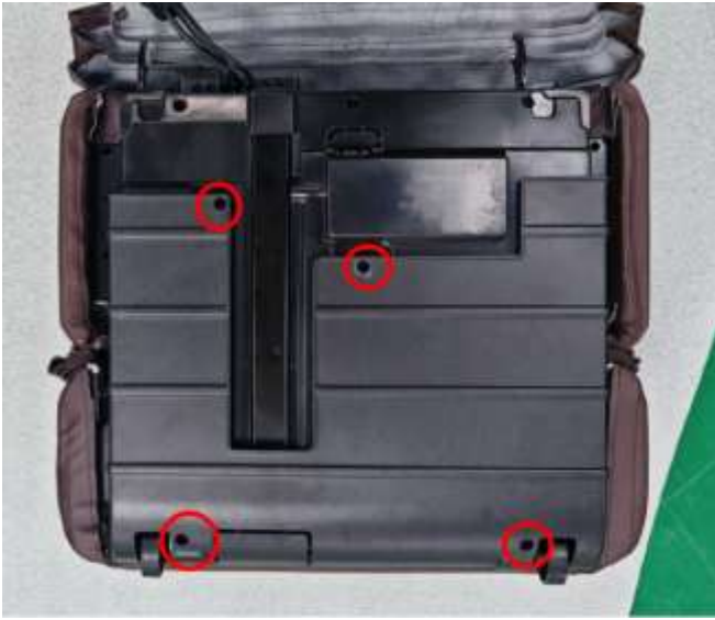
1. Remove the 4 screws and remove the cover plate
