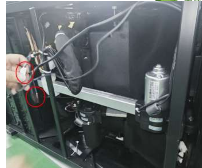
3.Disconnect the flat push rod terminal
