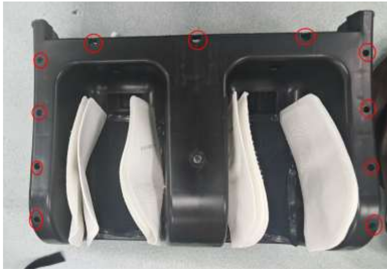
16. Remove 11 screws and separate the injection molded parts
