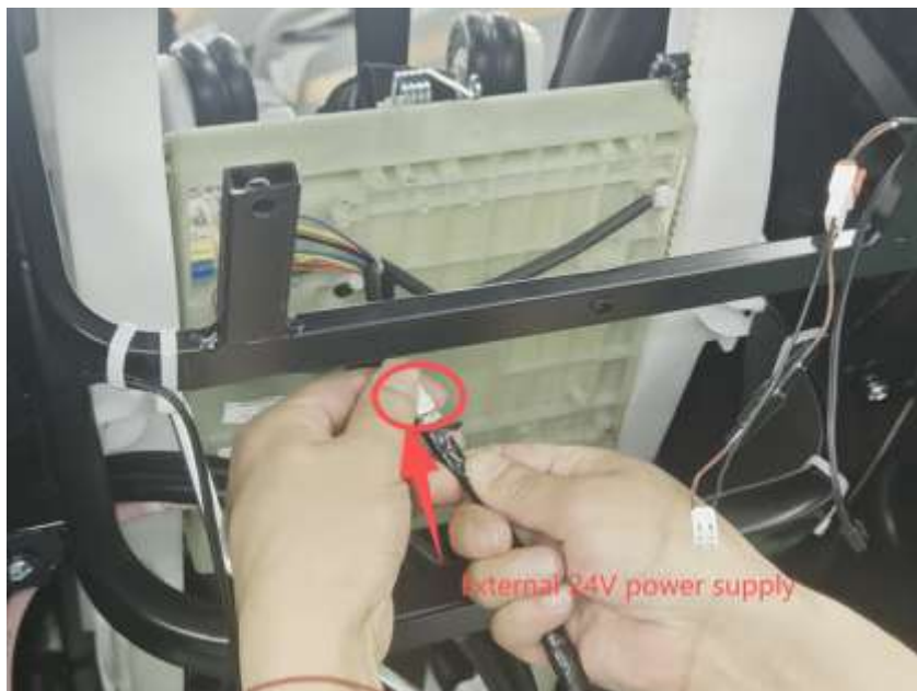
13. The terminals are externally connected to a 24V power supply to enable the movement to go up or down
