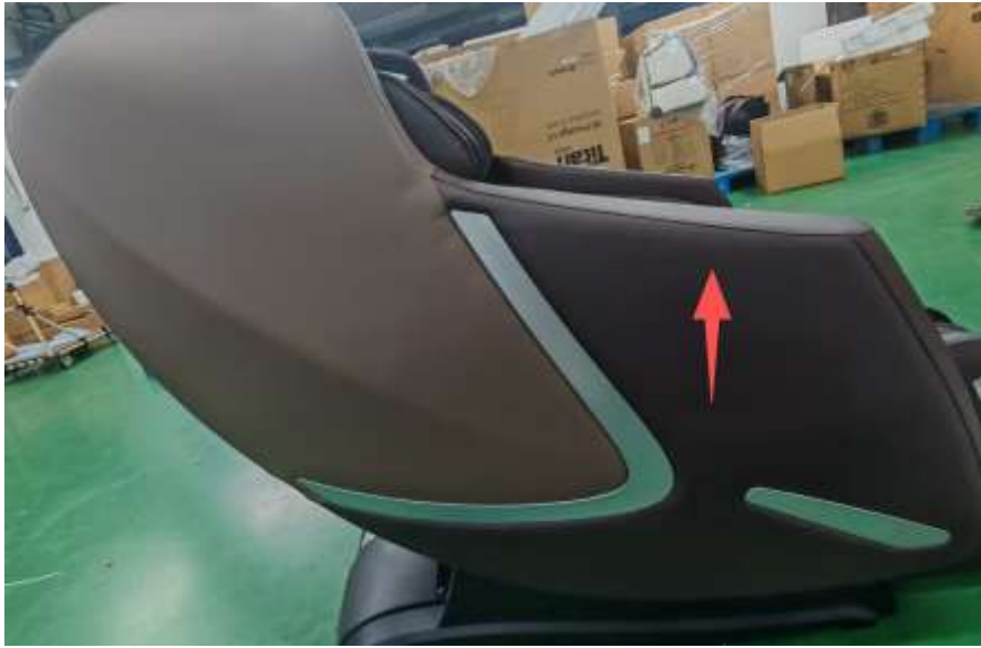
10. Pull out the side panels upwards
