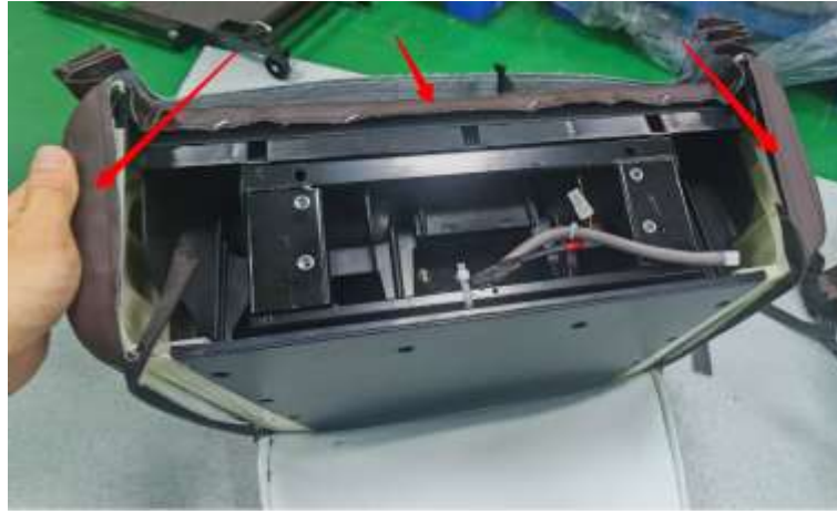
14. Remove the lower calf holster
