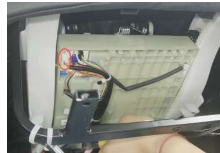
12.Disconnect the white two-core terminal
