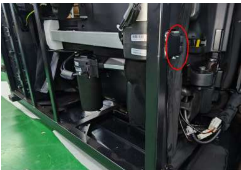
4.Pull off the cotter pin and remove the lower pin shaft
