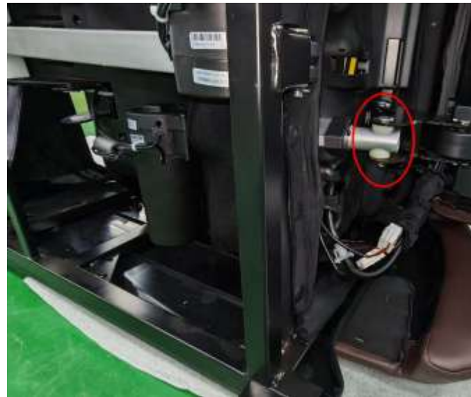
5.Pull off the cotter pin and remove the lower pin shaft
