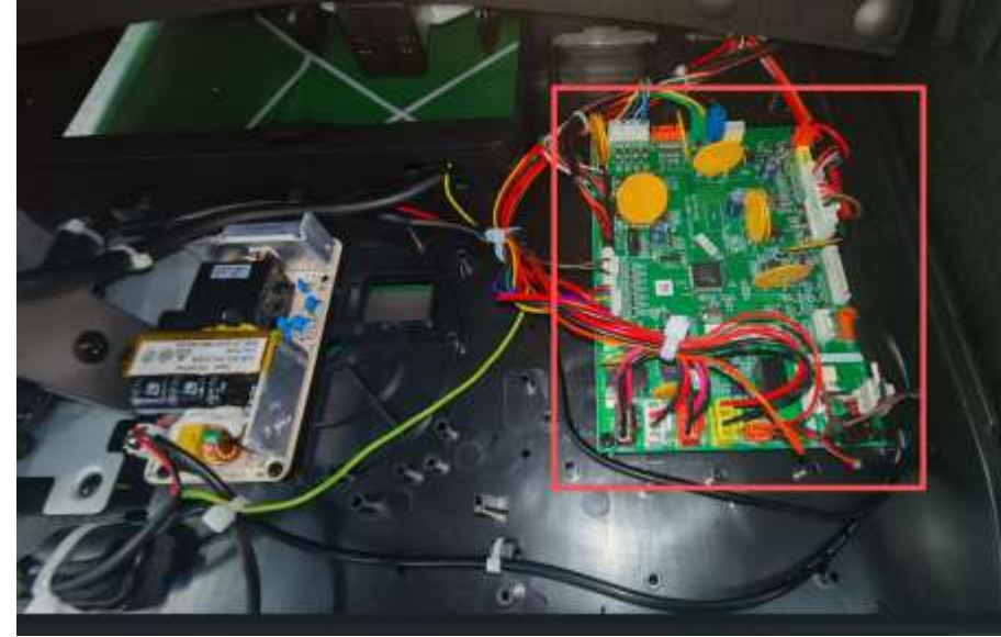
2.Disconnect the terminals and remove the 4 screws
