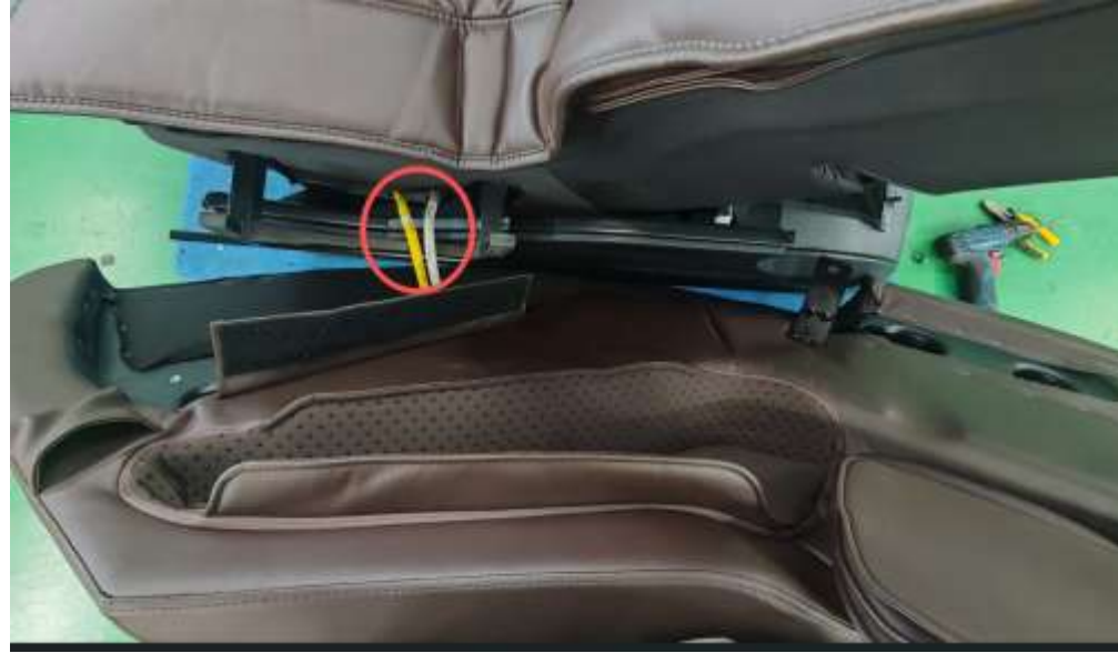
8. Disconnect the air pipe
