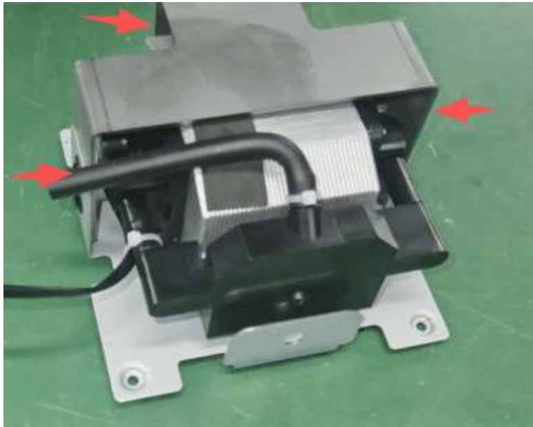
4.Remove 5 screws on three sides of the iron frame
