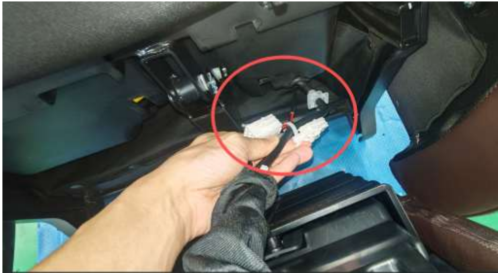
3.Cut off the tie buckle and disconnect the terminal and air pipe
