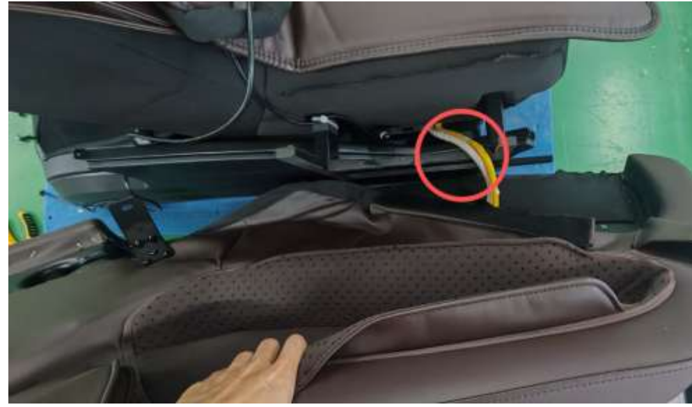
11. Disconnect the air pipe
