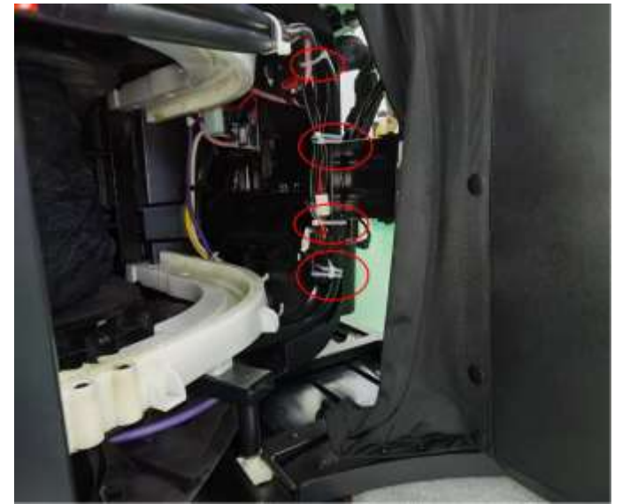
6.Cut off the tie
