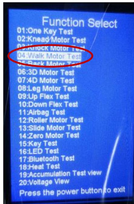
3. Enter background mode and choose walk motor test to run the mech until it stops at the top position.
