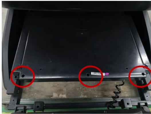
1. Unscrew the 3 bolts on the top cover and 3 bolts on the internal cover
