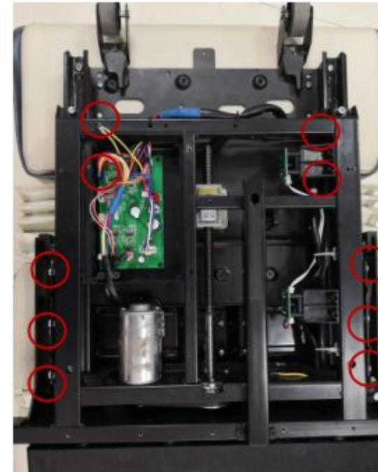
3. Unscrew the 6 bolts holding the extension unit, then remove the left 4 screws.
