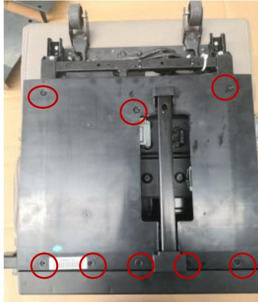
2. Unscrew these 7 bolts on the bottom cover board.
