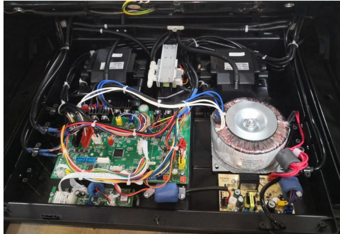
2. You may replace: main board pcb, user connecting pcb, power board pcb, transformer, air pump and air valve.
