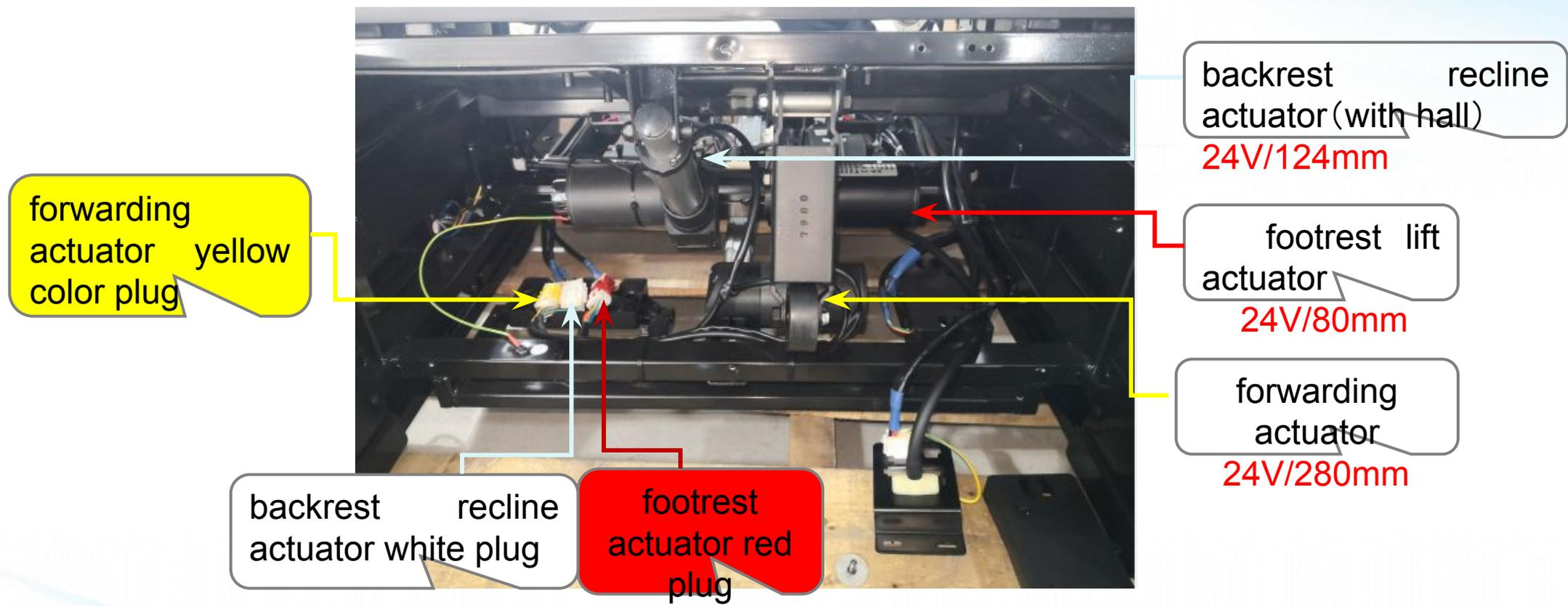
Remove the front and back cover board , unscrew the bolt at the front and back of actuator and unplug the connectors.
