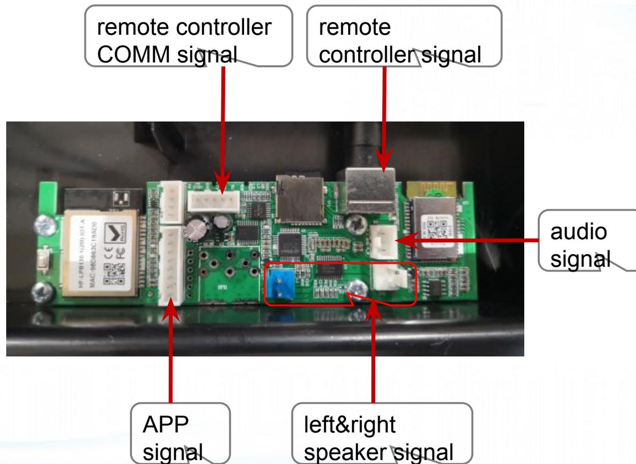
2.3 Footrest mainboard connector diagram
