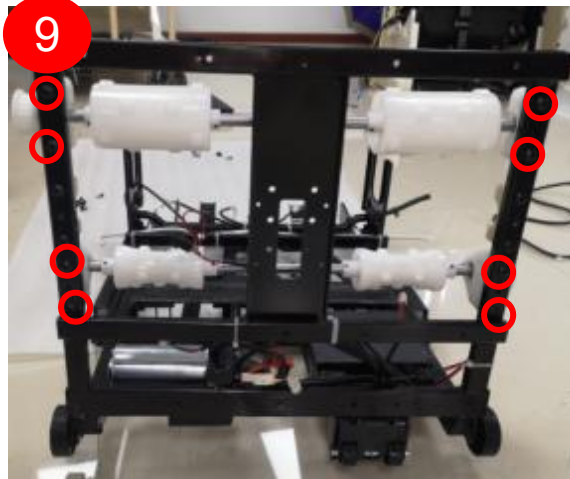
remove the screws fixing the middle roller
