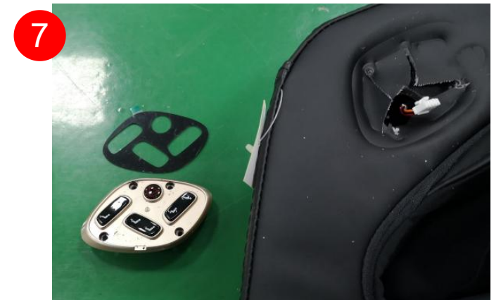
7 disconnected the terminal and remove the control
