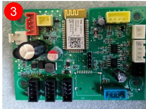
3 disassemble Bluetooth PCB
