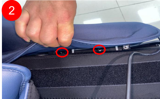
remove 2 screws, remove left side seat
