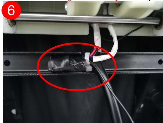
cut the heat shrinkable sleeve
