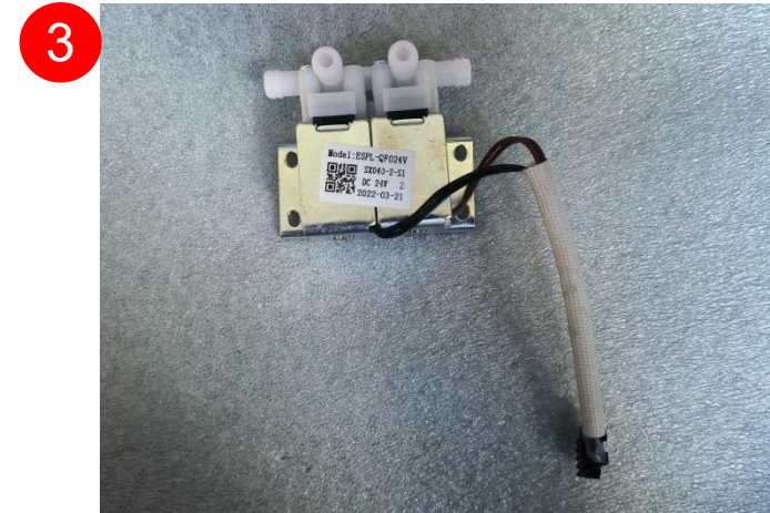
3 remove the air valve
