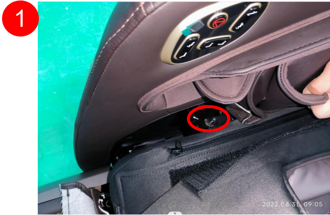
remove the screw of right side panel
