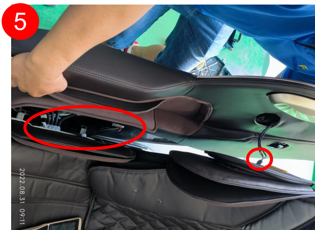
cut cable, discontent terminal and air hose
