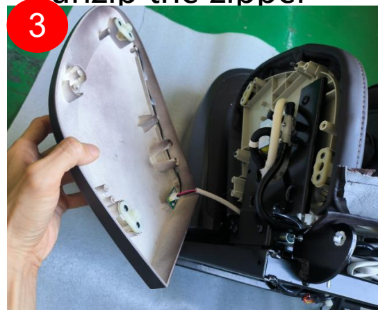
3 disconnected the terminal
