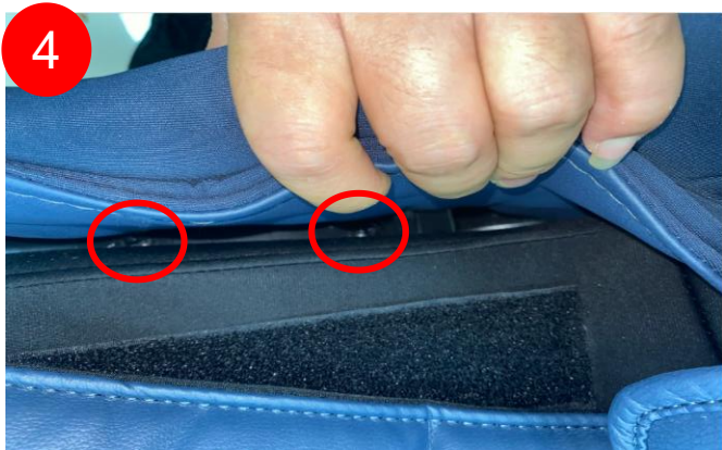
remove 2 screws, remove right side seat
