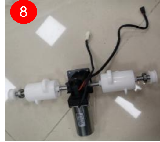
remove the middle roller unit
