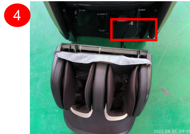
disconnected the terminal and air hose, remove the legrest
