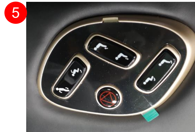
5 Pry off the key board assembly along the edge
