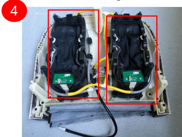
remove the screws fixing the cover
