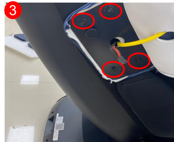
remove 4 screws, remove right shoulder unit
