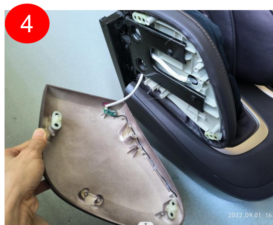
3 disconnected the terminal
