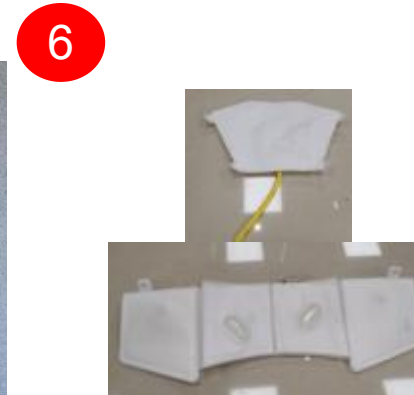
remove lower legrest and we can replace the air bag
