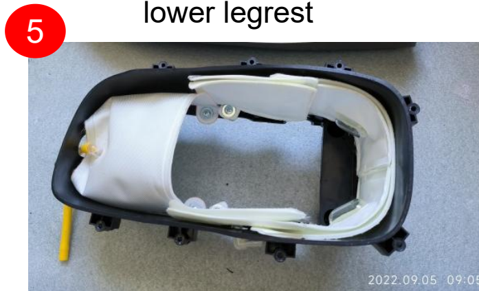
remove lower legrest and we can replace the air bag
