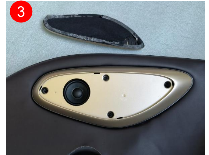
Pulling out trim,remove 4 screws
