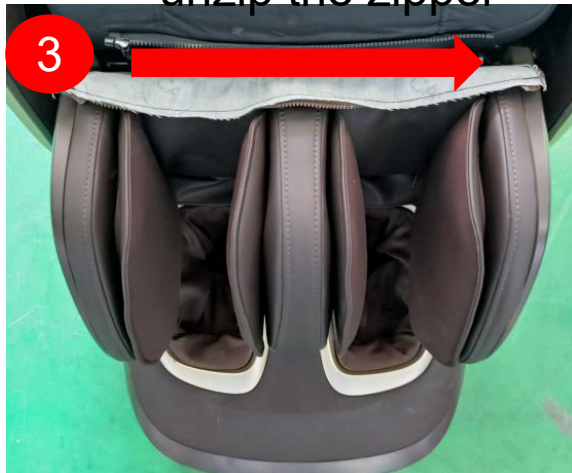
Remove the legrest in the direction of the arrow
