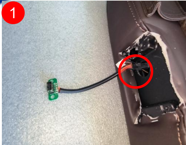
1 disconnected the terminal, remove the USB base PCB
