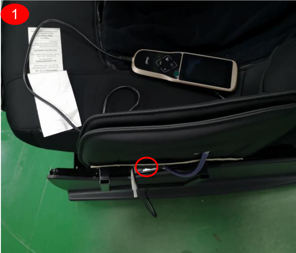
cut cable tie, discontent the terminal
