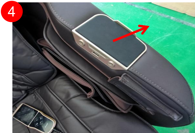
remove the silicone pad
