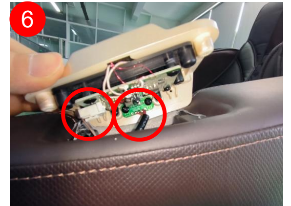
disconnected the terminal, remove 2 screws
