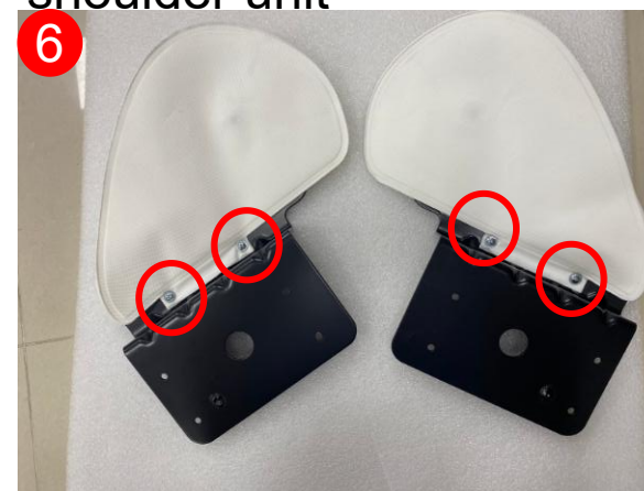
remove the screws and remove air bag
