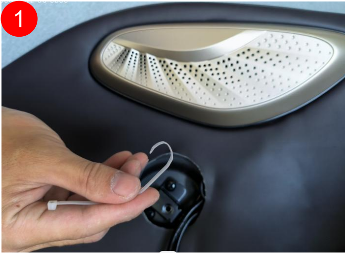
bending a small cable tie
