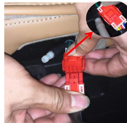
C、 Secure harness and air pipe
