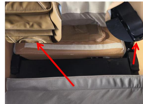
F、 Fasten protective cover and place leather
