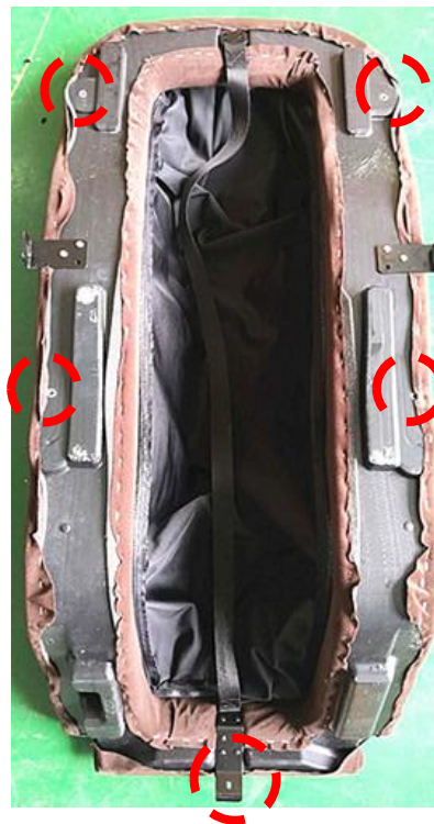
B、Remove the screw at one end of the bag strap and remove it from the massage hand, then you can take out the backrest frame
