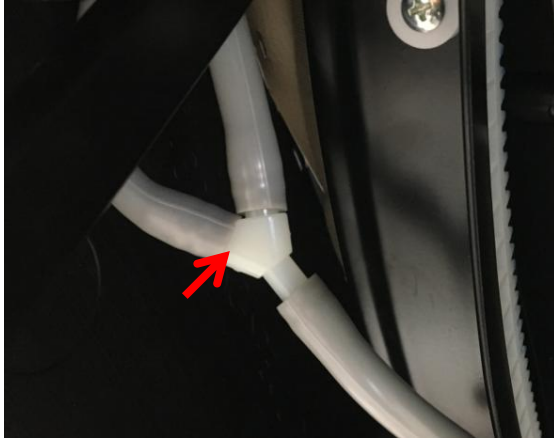
A , remove the back cover and separate the shoulder air bag air hose
