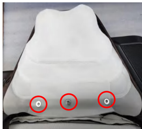
Remove the 3 screws securing the airbag.
