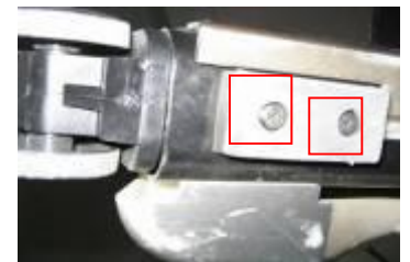
Screws securing the rubber support
