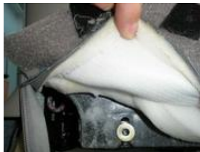
Screws fixing the lower part
