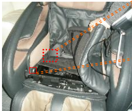
Screws (2pcs) securing the front panel
