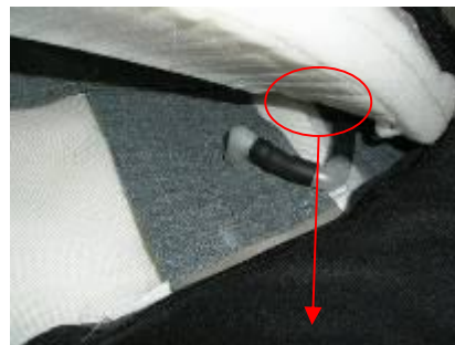
Pull out the hoses
