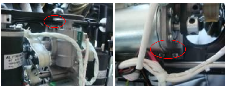
Screws securing the mechanism
