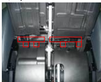
Screws(12pcs) securing the front panel
