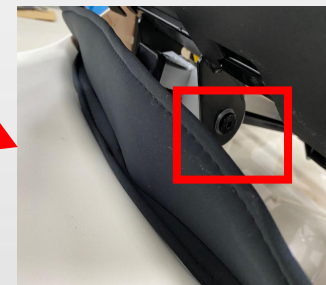
e. remove 2 screws, then remove the actuator
