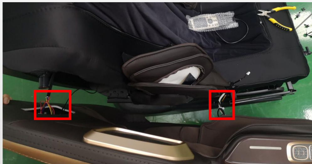
g. disconnected the terminals and air hose, remove right side panel
