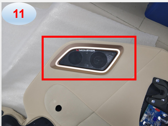
l. Tear off the horn net cover
