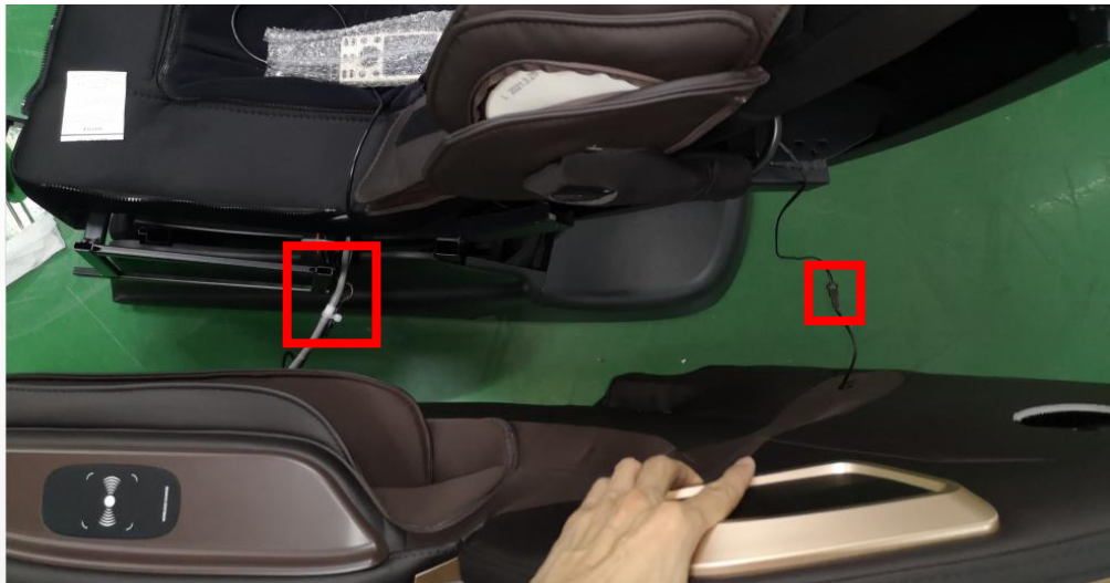
f. disconnected the terminals and air hose, remove left side panel
