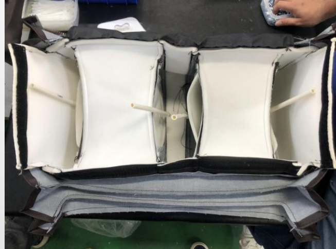
remove the cover and air bag
