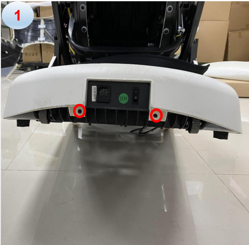
a. remove 2 screws and remove the cover
