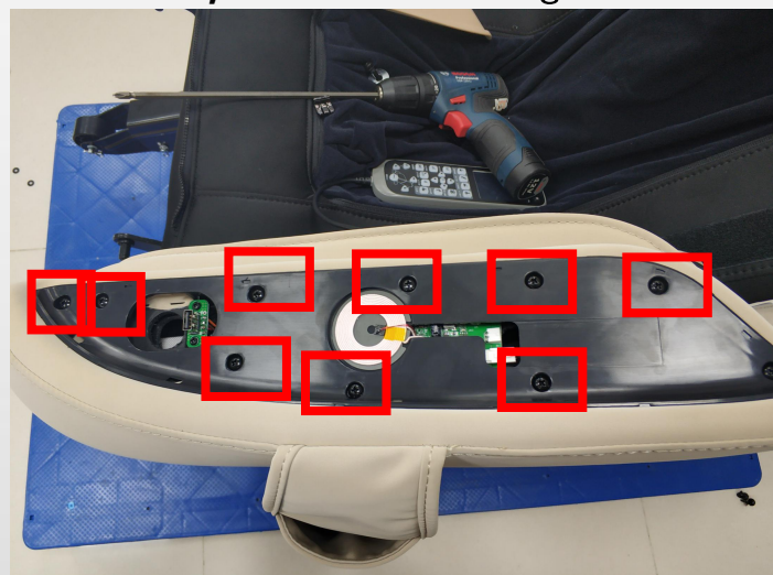
g.remove the screws
