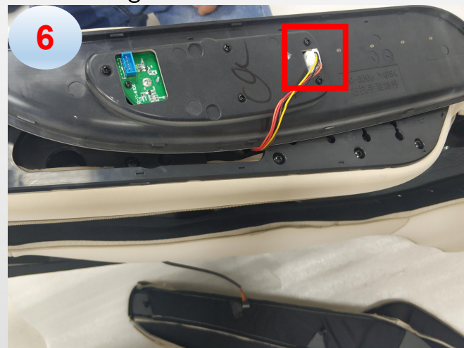
g. disconnected the terminals
