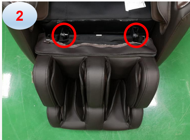
remove 2 limit baffles
