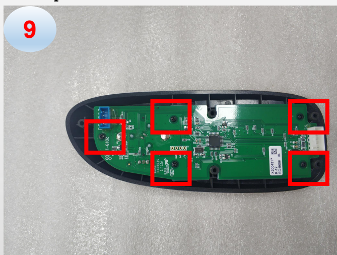
j. remove the screws and remove the PCBA
