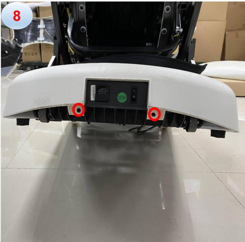
i. remove 2 screws and remove the cover
