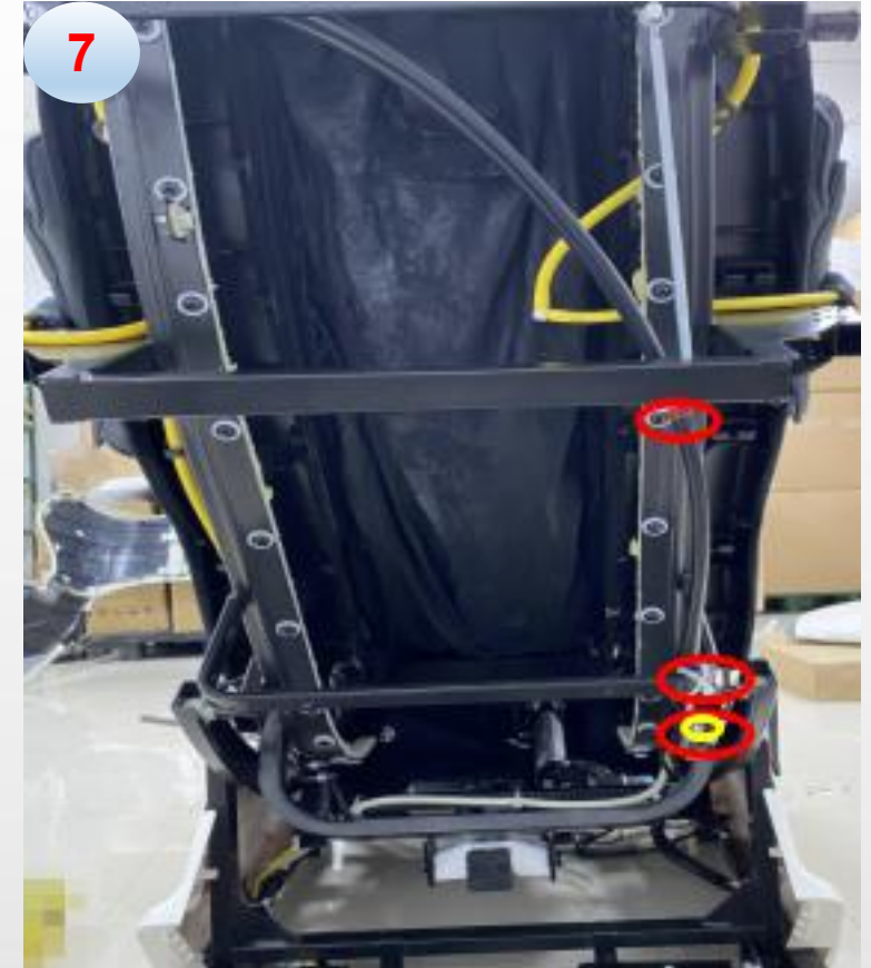
h. cut the cable tie and remove the screw fixing ground wire
