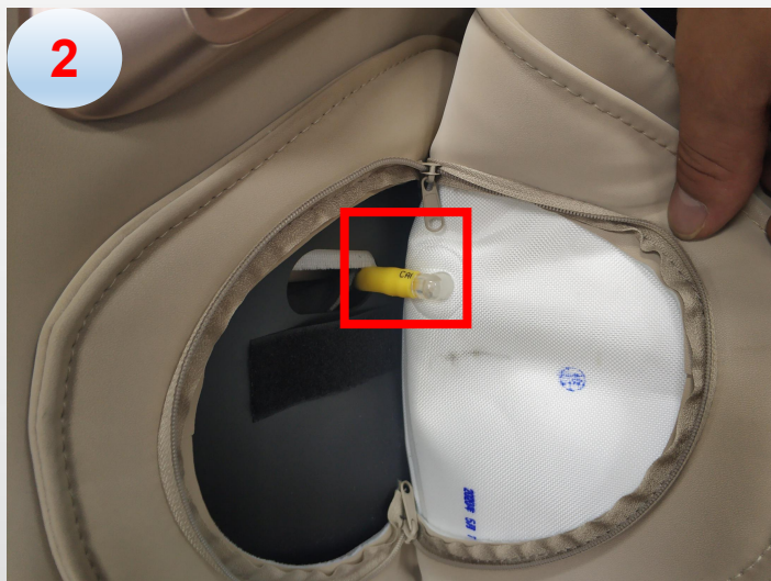
b. disconnected the air hose
