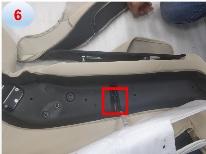
h. disconnected the terminal
