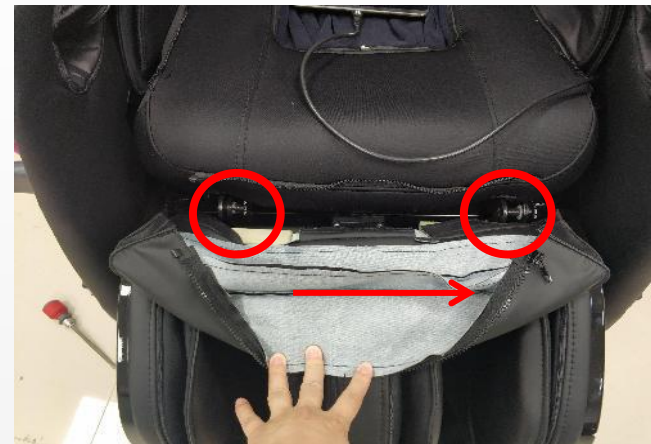
B. .Remove the blocking on both sides of the legrest
