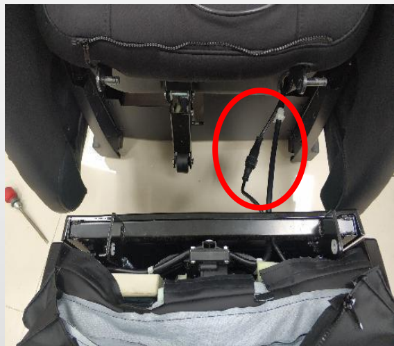
C. disconnect the terminal and air hose
