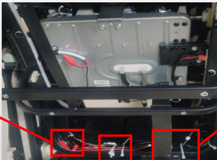
F.disconnect the terminals, remove the screw,cut cable tie,disconnect the air hose
