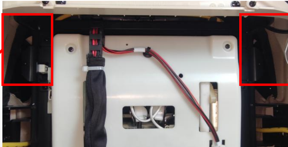
D.Remove the baffle both side
