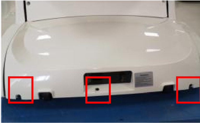
A.remove 3 screws, open the main PCB box
