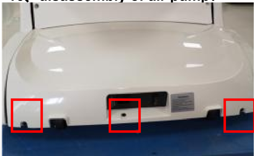
A.remove 3 screws, open the main PCB box
