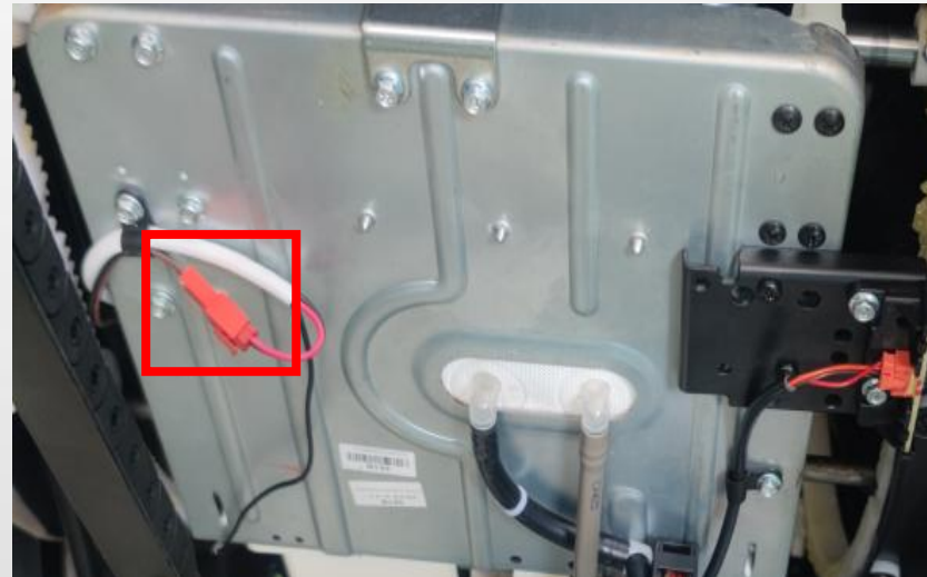
M.connect red terminal with a 24V power, mechanism go up
