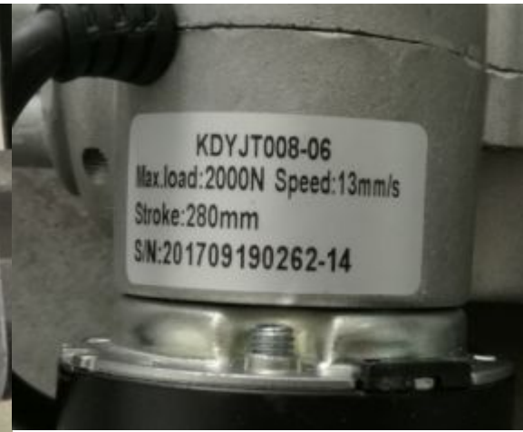
forward cylinder DC24V/280mm
