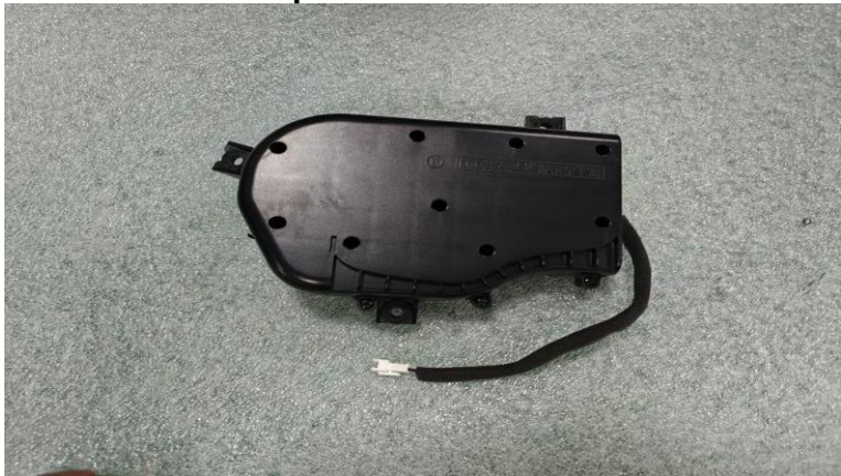
Remove the horn component
