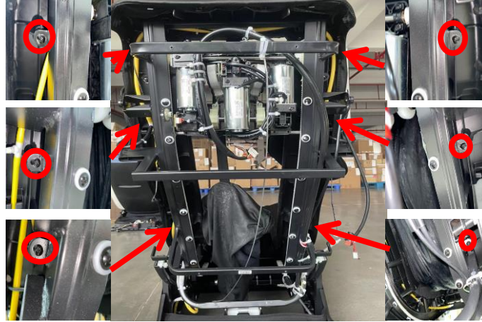
Remove the 6 screws securing the front backrest
