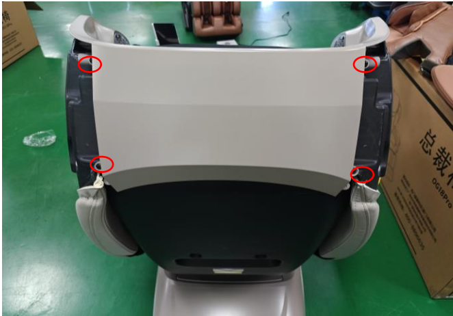
Remove the four fixing screws
