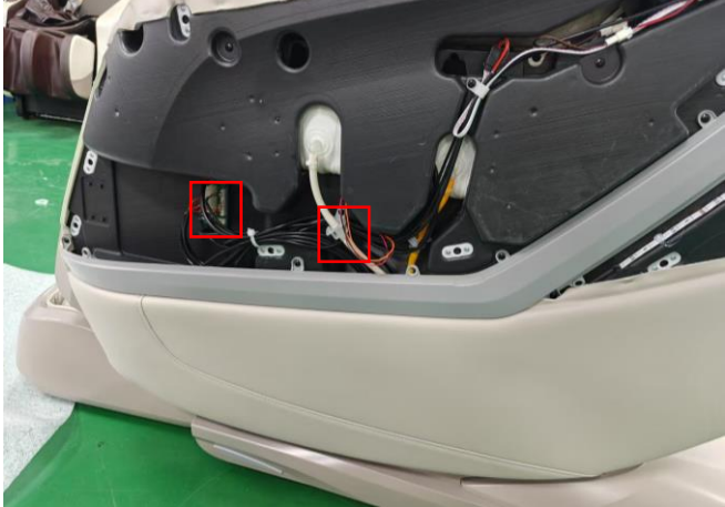
Unplug all connected terminals and air tubes, and remove the left side panel
