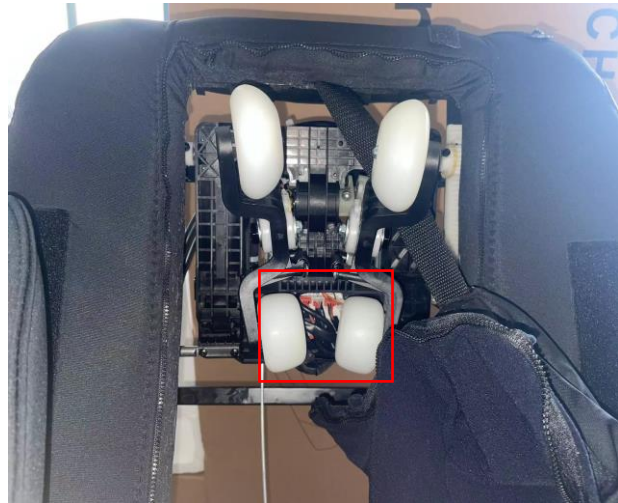
Remove all terminals from the adapter board of the movement
