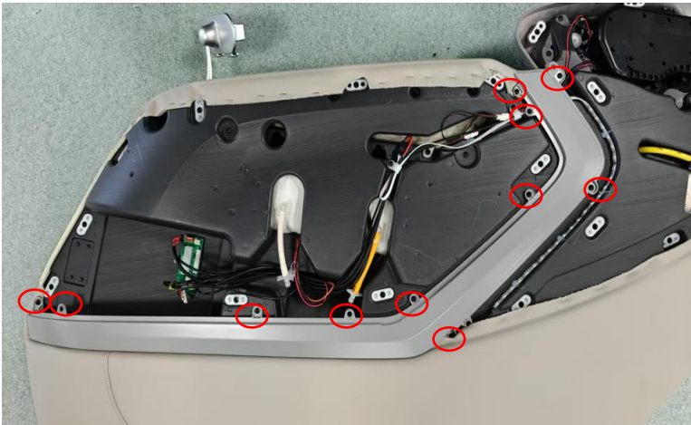
Remove the screws and remove the decorative parts
