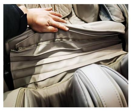
2. You can see the zipper of backpad. Unzip it and then you can take the backpad off. When you unzip the backpad, you can see there is connection to heating pad and airbag inside the backpad.
