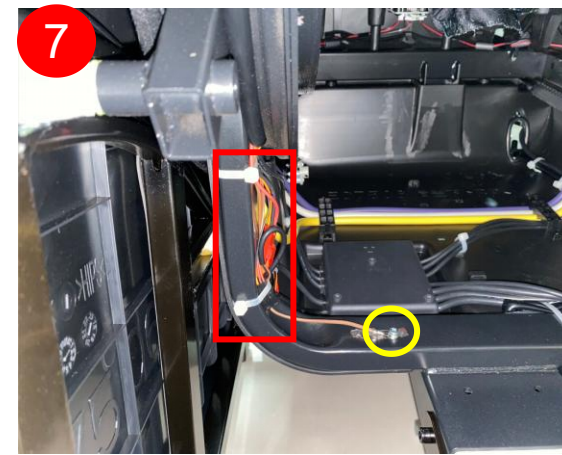
Cut off the buckle, pull out the terminal (marked in red), remove the ground screw marked in yellow, and take out the back stringing
