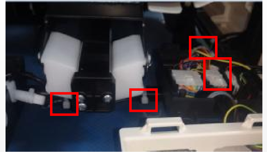
C.cut cable tie, disconnect the terminal
