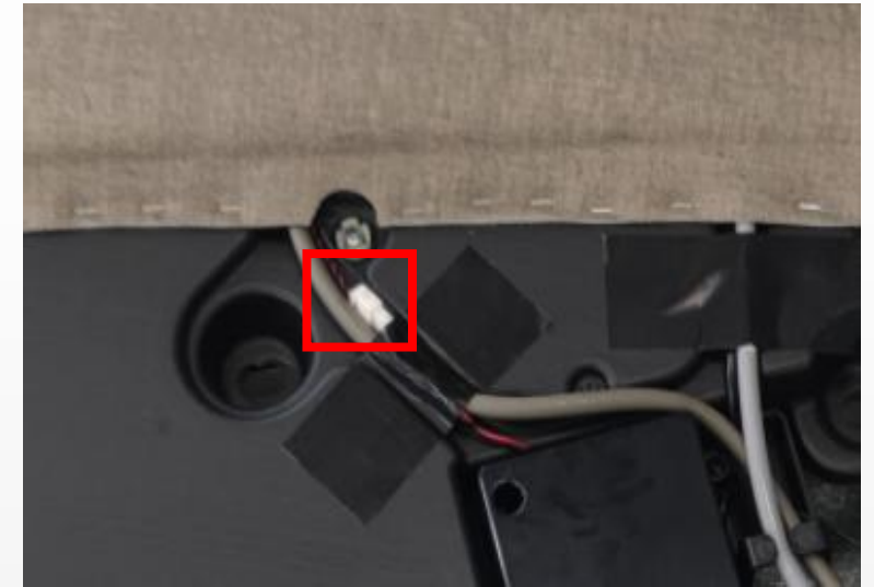
L. disconnect the terminals
