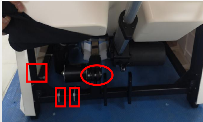
E.cut cable, remove the shaft
