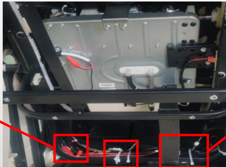
F. discontenent the terminals, remove the screw, cut cable tie, disconnect the air hose
