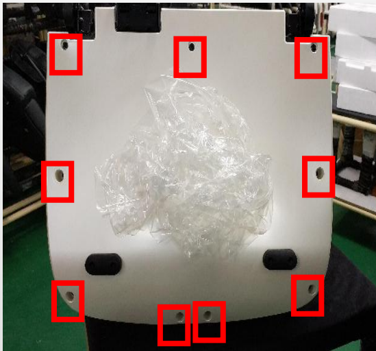
D. remove 9 screws
