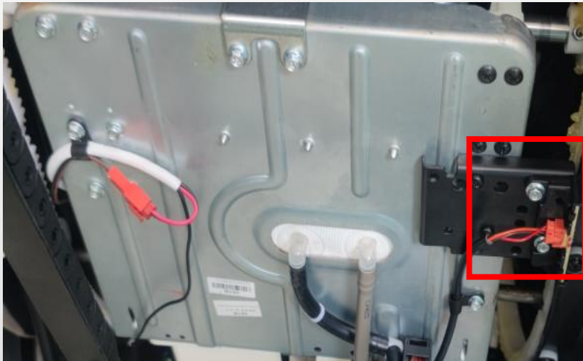
N.disconnect the, disconnect the air hose,remove the rack
