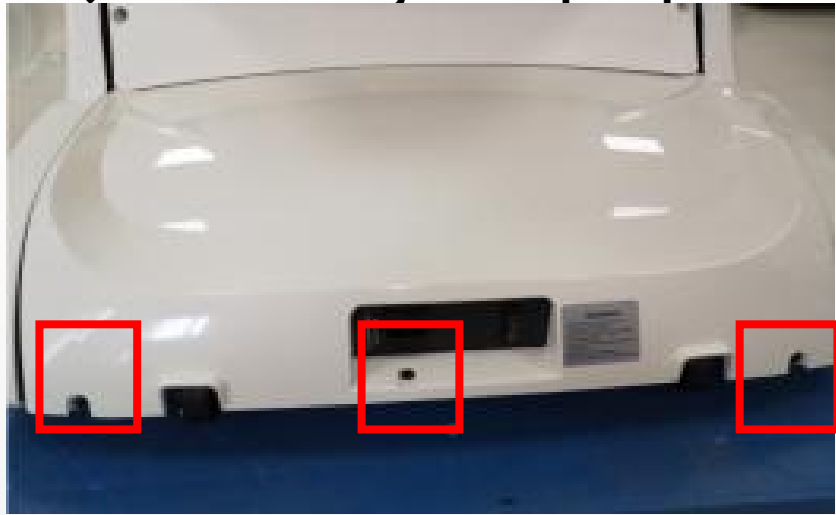
A.remove 3 screws, open themain PCB box
