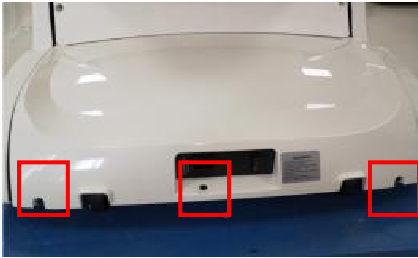
A.remove 3 screws, open the main PCB box
