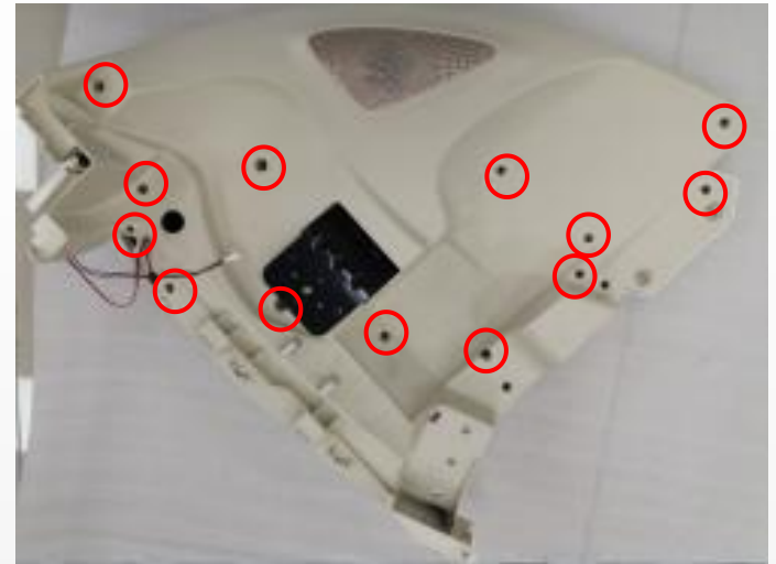
E.remove the screws
