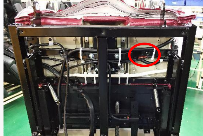
B. Cut off button, Unplug all terminals
