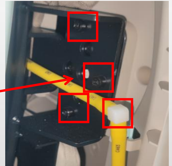
C. remove 4 screws
