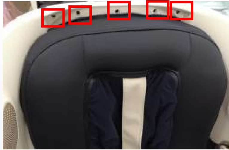
B. remove 5 screws
