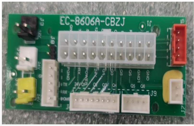
C.side panel switch PCB
