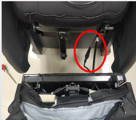
C. disconnect the terminal and air hose
