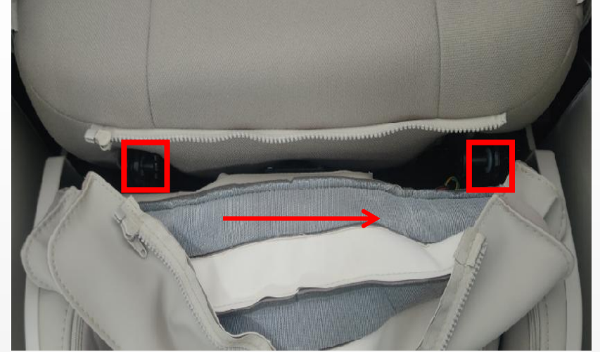
C.Remove the blocking on both sides of the legrest
