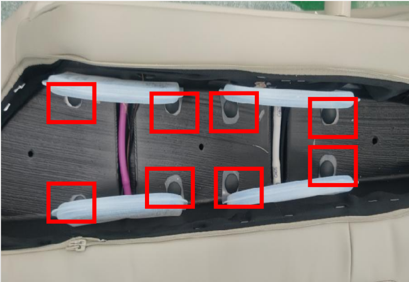
G. break open the cloth cover pin, disconnect the air hose
