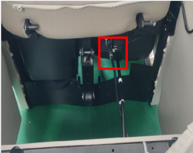
D.disconnect the terminal and air hose
