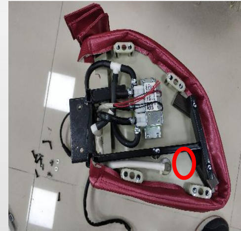
K. Pull out all the air pipes, All air bags can be replaced
