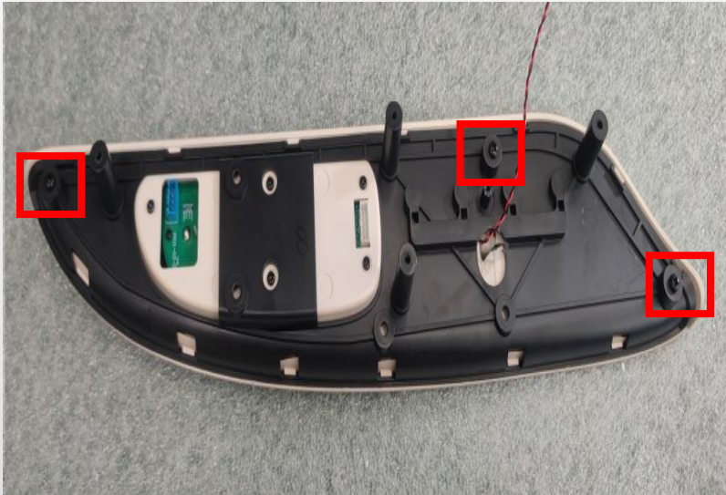
Q . remove 3 screws
