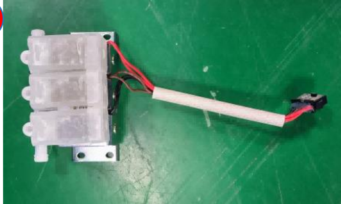
remove the 3-way air valves
