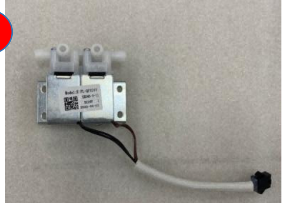
remove the 2-way air valves
