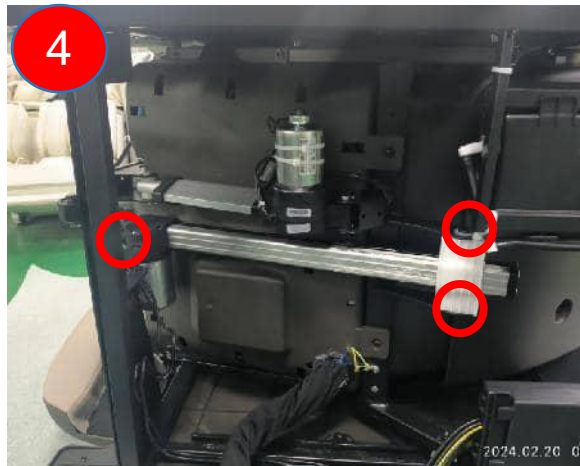
Remove the front pin and rear screw
