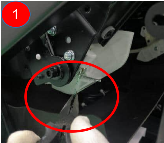
1 clamp the spring open with apointed nose pliers
