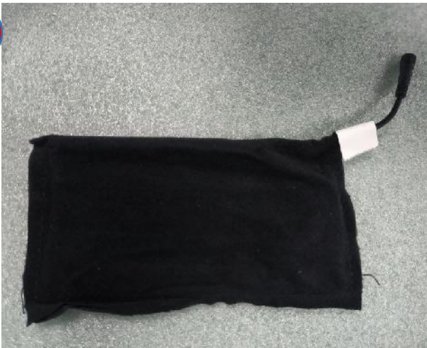
remove the seat heater
