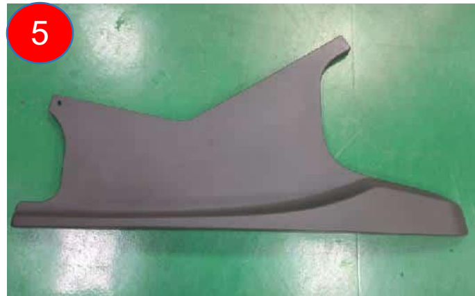
remove lower side panel
