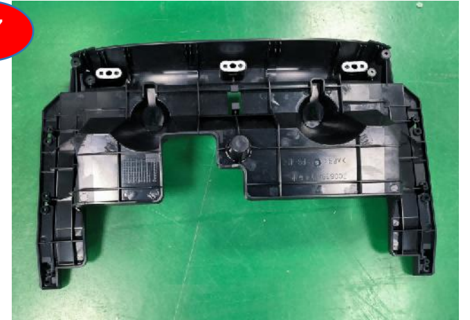
Remove the middle hood inner cover
