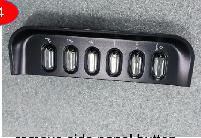
remove side panel button assembly
