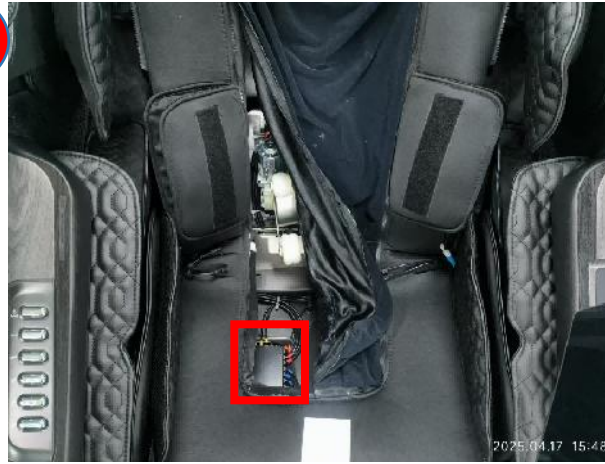
the position of under seat PCB
