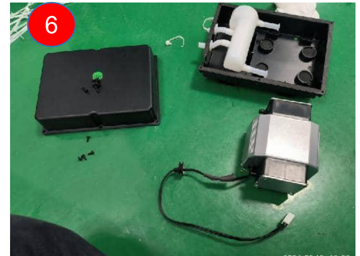
separate the air pump
