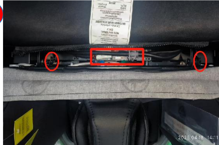
discontentthe terminal and air hose, remove 2 catch pins
