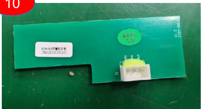
remove collision detection board
