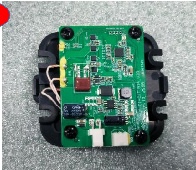
remove wireless charging unit
