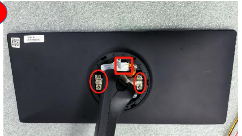
remove the screws, discontent the terminal
