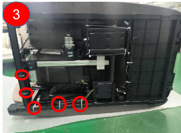
cut the cable tie
