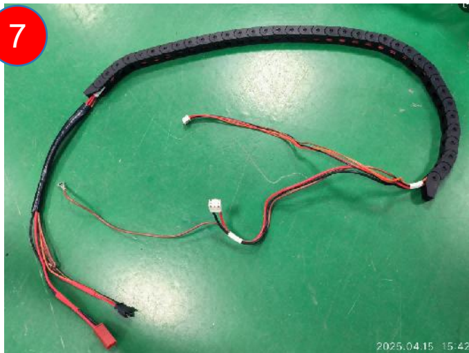
remove lower backrest cable
