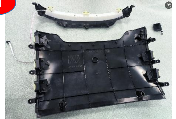
Separate the middle hood cover
