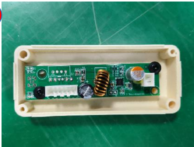
remove the USB charging PCB
