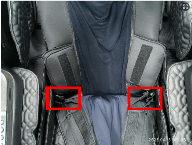
disconnect the terminals
