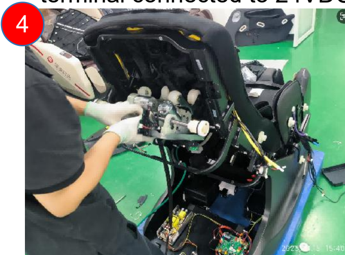
4 remove lower gear box
