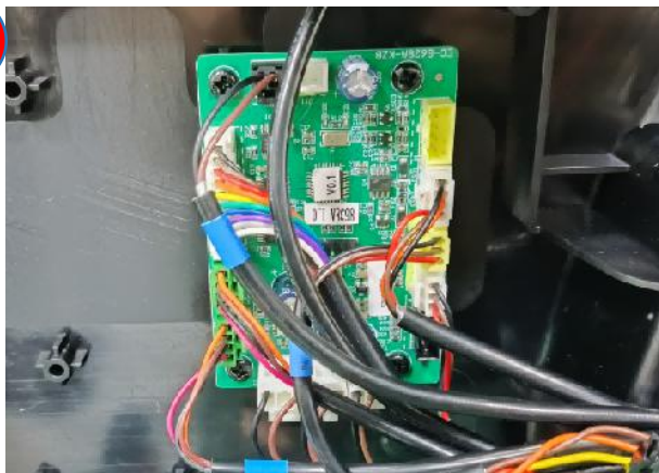
remove the screws, discontent the terminals
