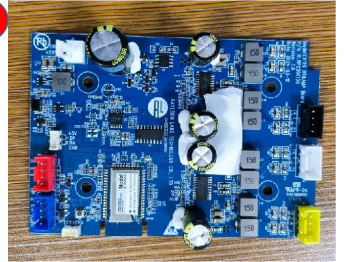
remove Bluetooth PCB
