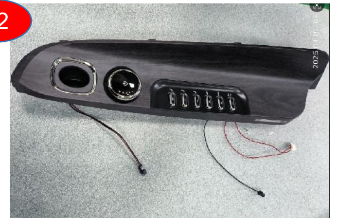
remove the arm cover unit
