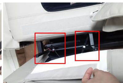
断开气管和端子 Disconnect air hose and terminal
