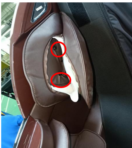
remove 2 screws of the right shoulder
