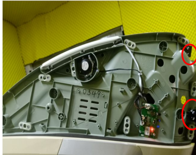
remove 4 screws left side
