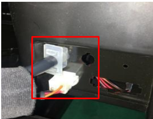
discontent the terminal and air hose
