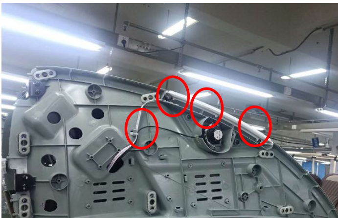
cut the cable tie, remove 3 screws
