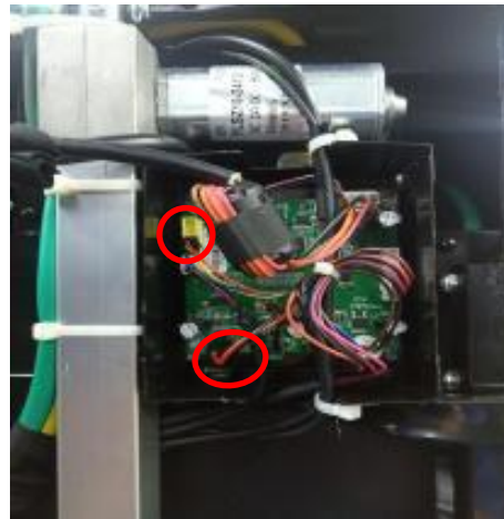
disconnect the 2 terminals
