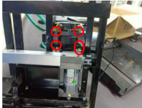
remove the other 4 screws
