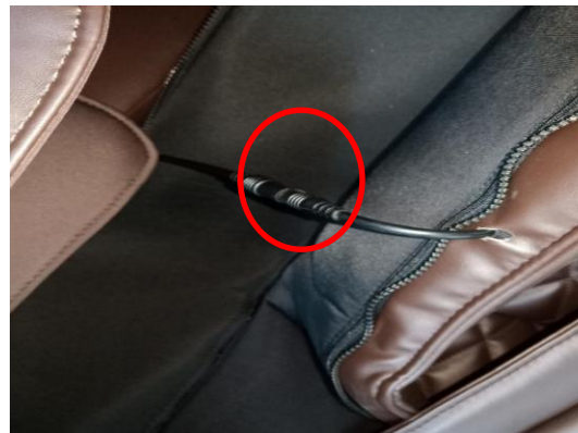
discontent the heater terminal
