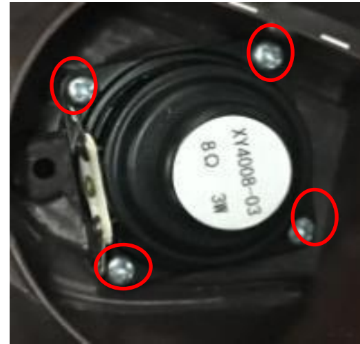
Remove four screws and replace the horn
