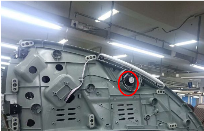
Disconnect the right horn cable
