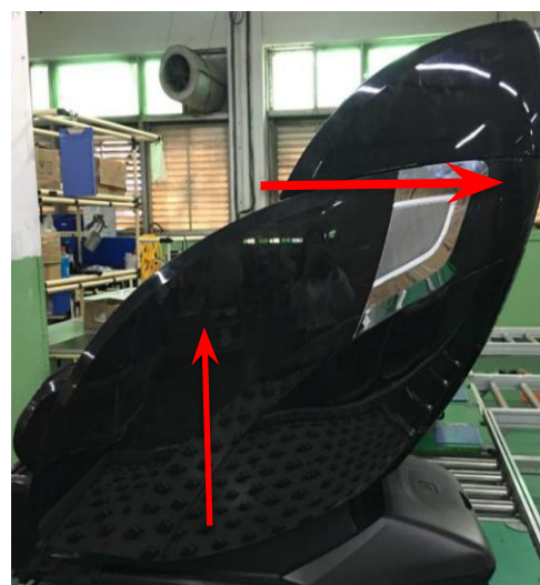
lift up the side panel, move the side panel backward
