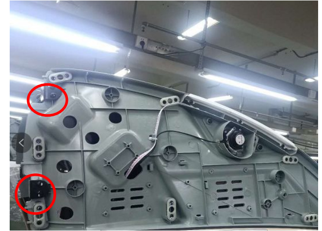
remove 4 screws right side
