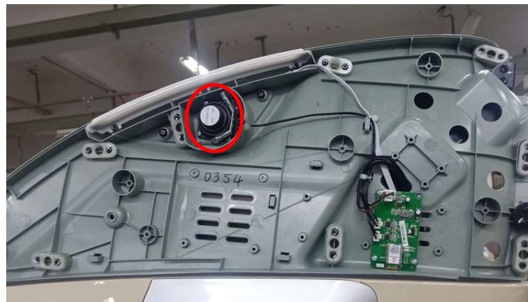
Disconnect the left horn cable
