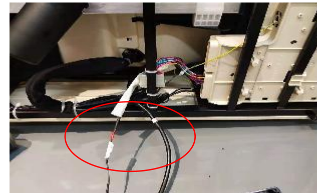
C.disconnect the air hose and terminal
