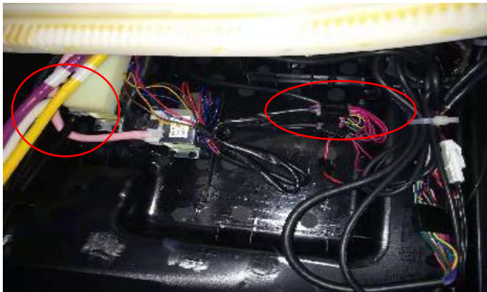
C.disconnect the air hose and terminal
