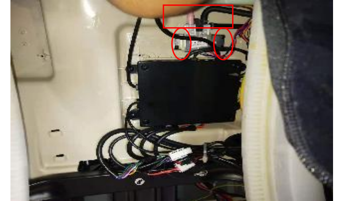
C.remove the screws, disconten the terminals, remove air valve
