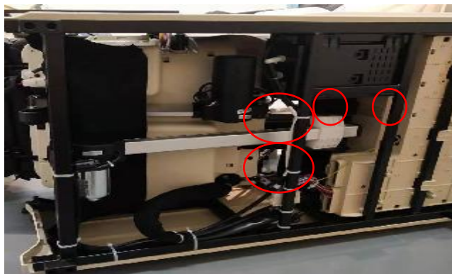
B.cut cable tie, remove 2 screws
