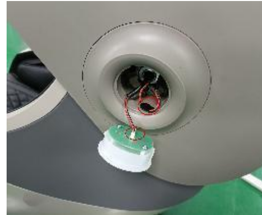
B. Disconnect the lamp shade terminal, Remove the lampshade
