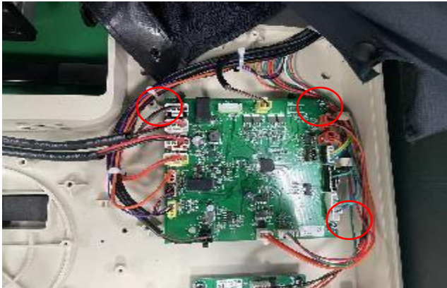
D.discontent the terminals and screws
