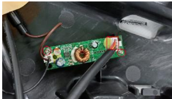
E. Disconnect the port and remove the 2 screws
