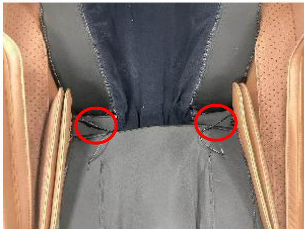
B.Unscrew and unplug 2 heating terminals
