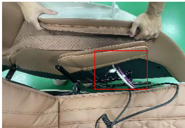
B. discontent the terminal and air hose
