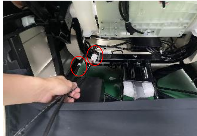
H.disconnect the terminal and air hose
