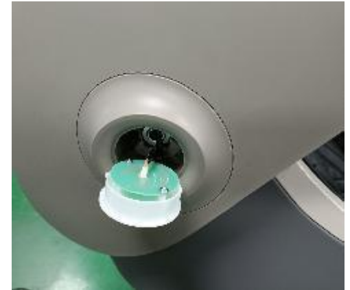
B. Disconnect the lamp shade terminal, Remove the lampshade
