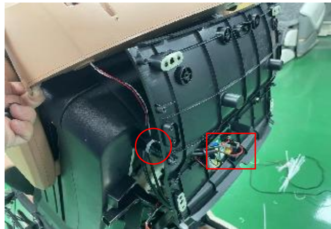
E.cut the cable tie, discontent 2 terminals
