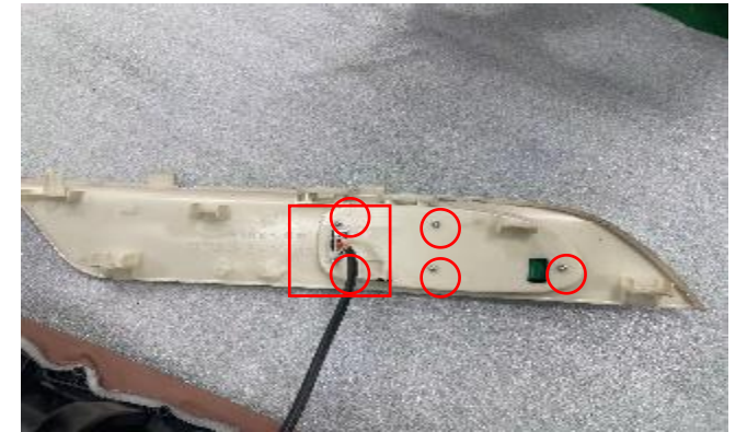
F.remove 5 screws, discontent the tterminal
