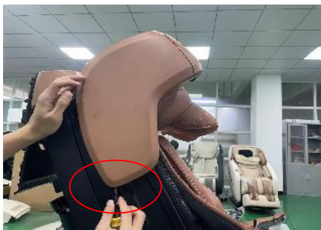
J .open the cover with a “—” screwdriver
