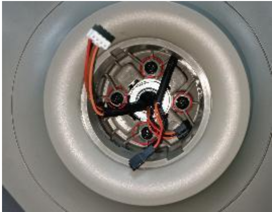
C. Remove 4 screws on the left and right
