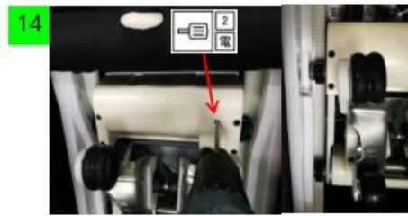
14. Remove gear box away from the baffle of the left and right guide rails with the electric screwdriver 2.
