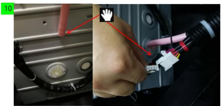
Back line and trachea connect with external wiring air bag of gear box
