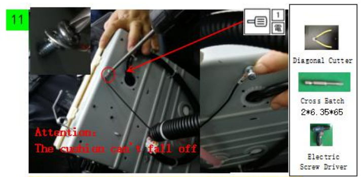
Lock the ground wire of gear box to the gear box with the electric screwdriver 1.
