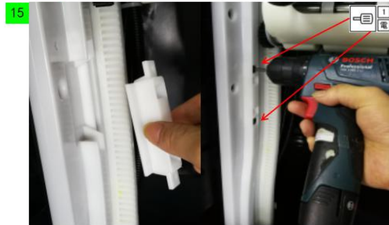
15. Move the baffle of the left and right to guide rails with the electric screwdriver 1.
