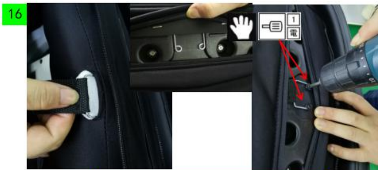
16. Pass the barb through the elastic cloth, lock two screws with screwdriver 1.
