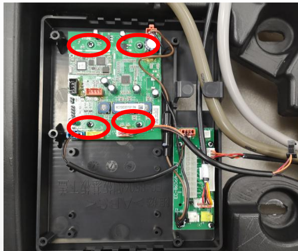
G. disconnect the terminals, remove 4 screws
