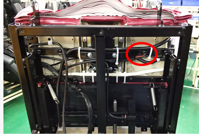
B.Cut off button,Unplug all terminals
