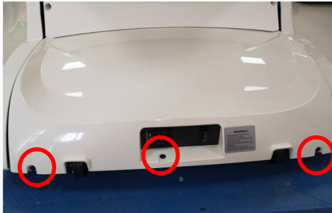
A.remove 3 screws, open themain PCB box
