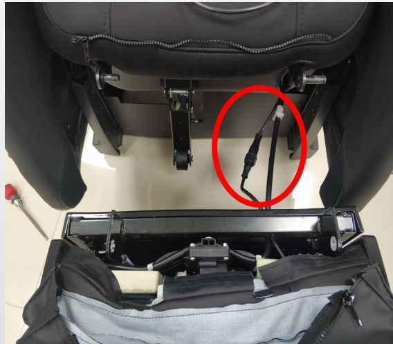
C. disconnect the terminal and air hose
