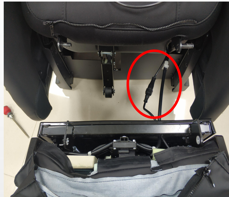
B. disconnect the terminal and air hose
