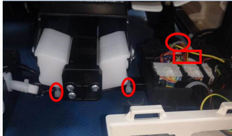
B.cut cable tie, disconnect the terminal
