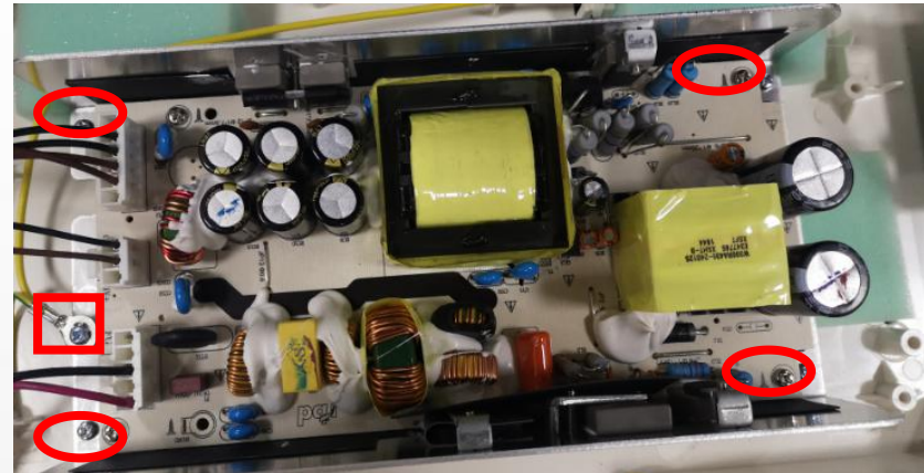
disconnect the terminals, remove 5 screws
