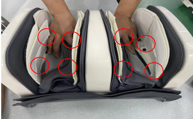
Remove a total of 8 screws on the left and right sides
