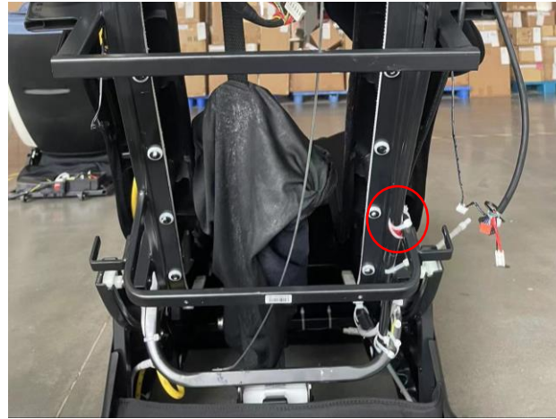
Cut off the backrest wire cable tie
