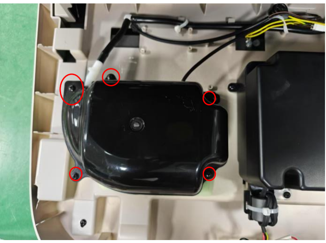
Remove 5 screws and take off the cover
