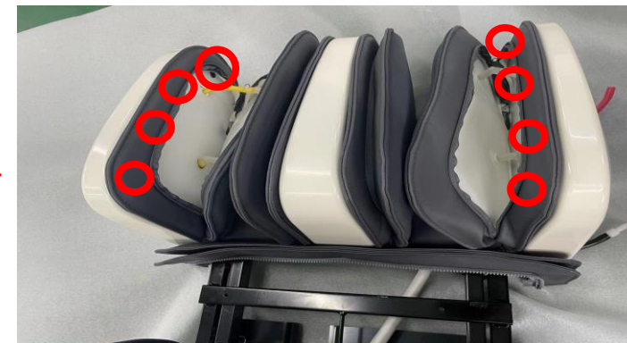
Remove a total of 8 screws on the left and right sides
