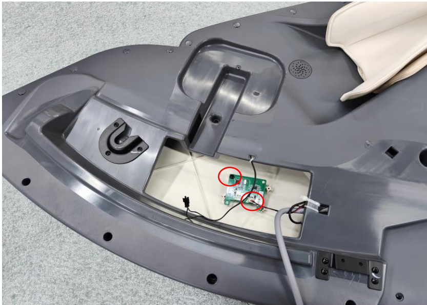
Remove one screw and disconnect one terminal
