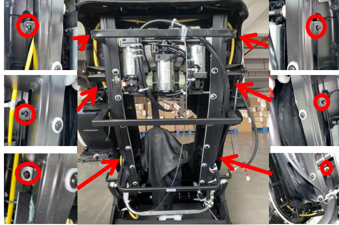
Remove the 6 screws securing the front backrest
