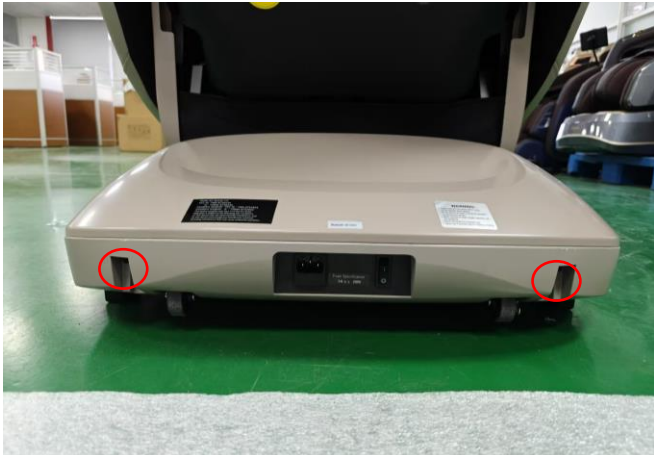
Remove 2 screws and take off the top cover of the center box
