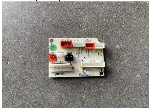
Remove the adapter plate of the movement
