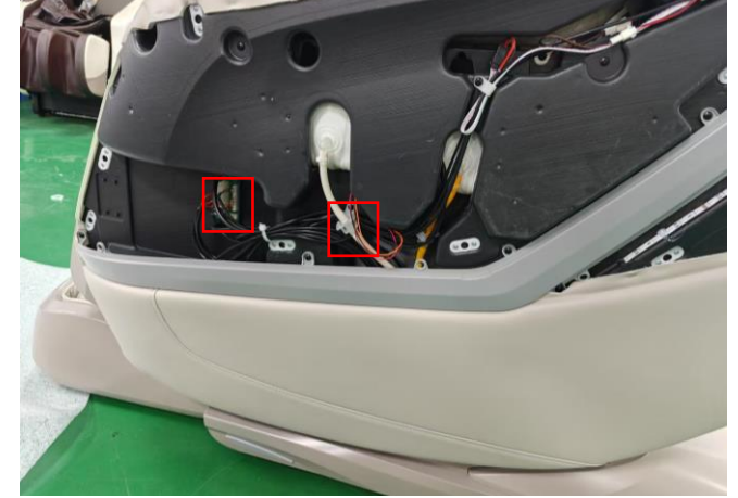
Unplug all connected terminals and air tubes, and remove the left side panel
