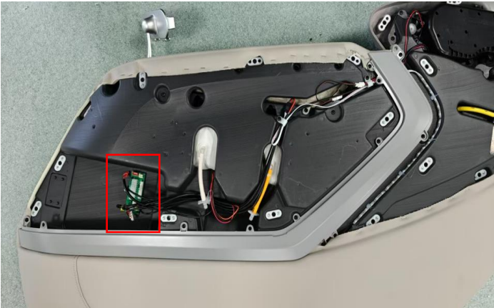
Unplug the terminal and remove the side panel adapter board
