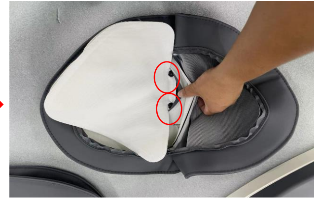
Remove the two screws on the right shoulder
