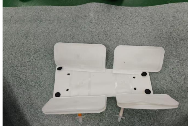
Remove 4 screws, cut off the zip ties, and unplug the terminals
