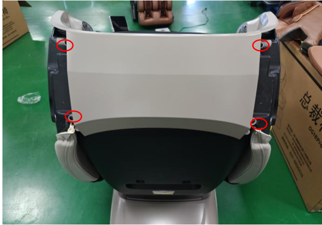
Remove the four fixing screws
