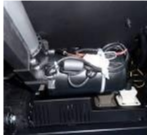
抬起小腿拆下前档板,之后定位图中三个位置,除下它们即可(建议先拆上方销轴以方便拆底部销轴) Pull-up the legrest and disassembly the plate washer then location map of three position, (moving the top of pin first)
