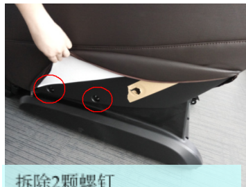
拆除2颗螺钉 Demolition of two screws
