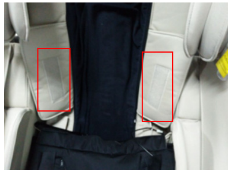
披风与靠背的拉链 the zipper fixing the pad and the backrest
