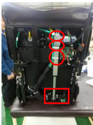
cut the cable tie, take down the shaft
