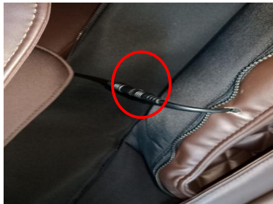
discontent the heater terminal
