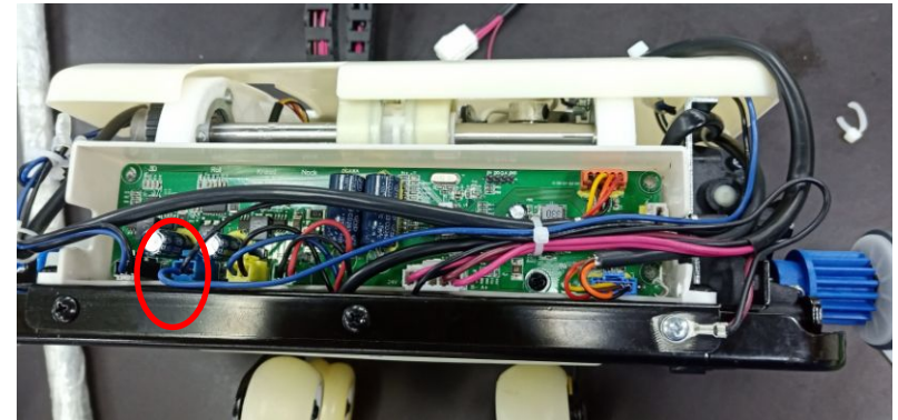
find out the blue terminal, let mechanism go down with 24VDC power
