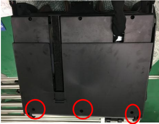
remove 3 screws fixing the rear cover and take it down
