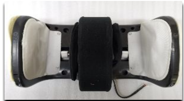
E. Separate the calf kneading assembly
