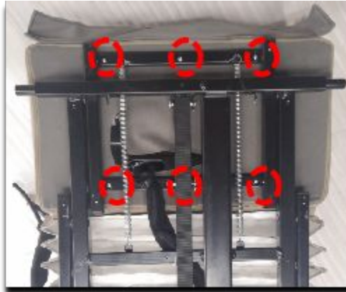
B. Remove the 6 screws in the red ring of the calf steel frame
