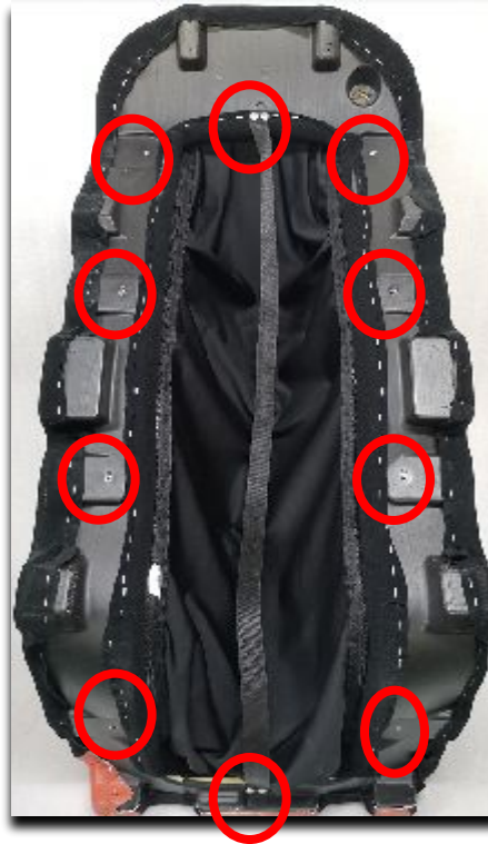
B. Remove 10 screws in the red circle
