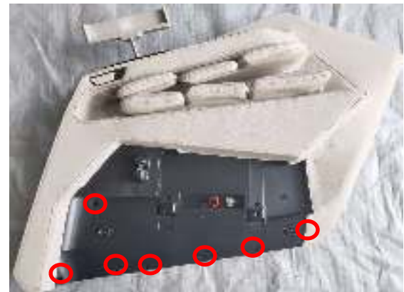
M6×30 hexagon socket head cap screw + φ6 flat washer
