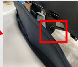
4 e. remove 2 screws, then remove the actuator
