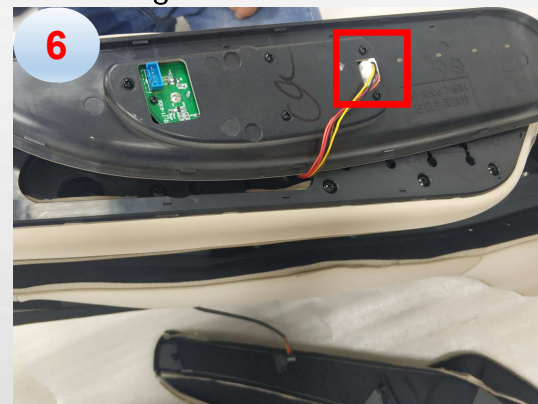
g. disconnected the terminals
