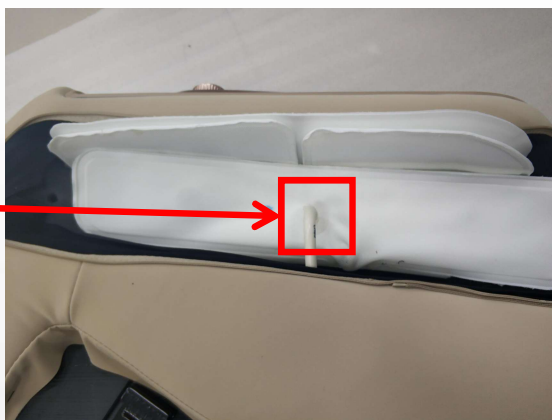
e. remove the screws, disconnected air hose, remove air bag
