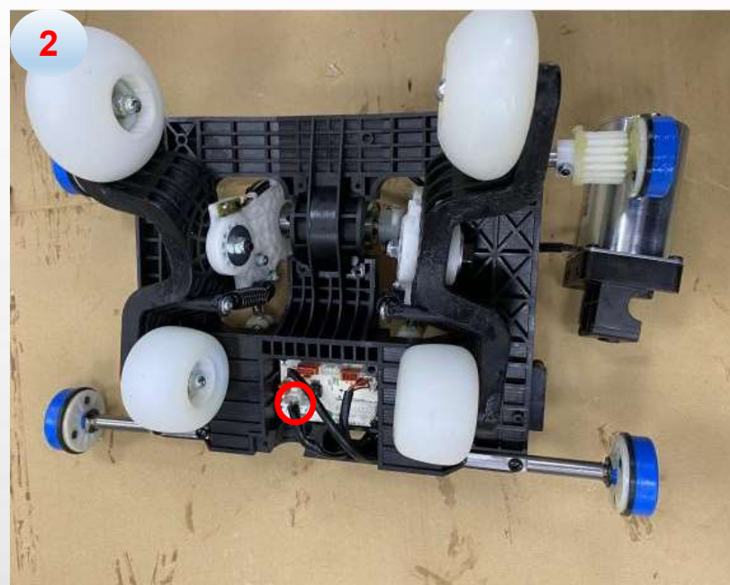
b. disconnected 2 terminals of the motor
