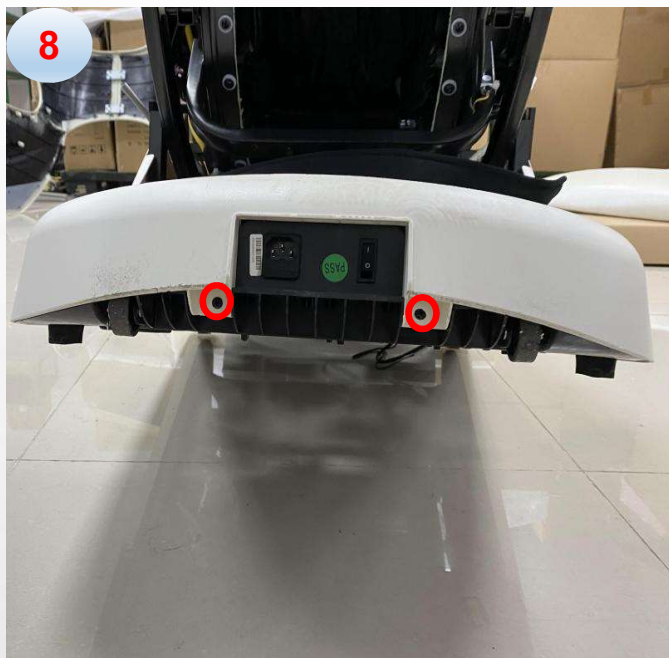
i. remove 2 screws and remove the cover
