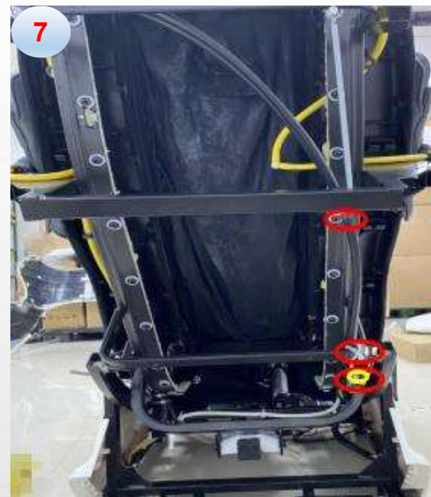
h. cut the cable tie and remove the screw fixing ground wire
