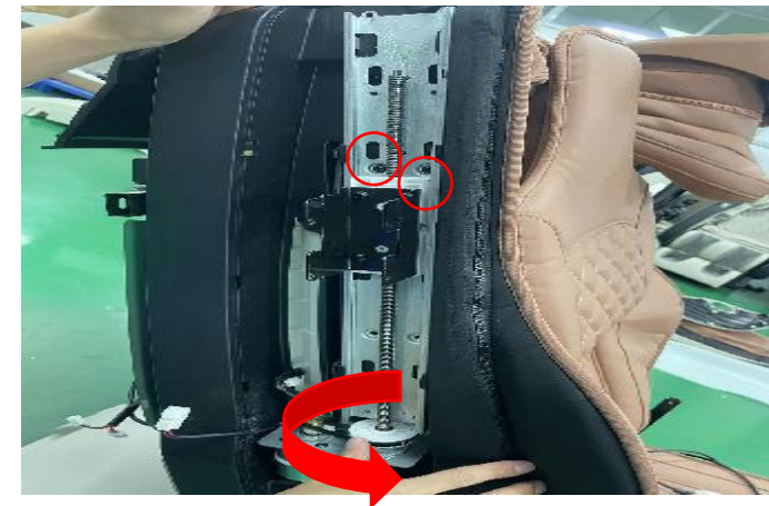
R .Rotate the motor counterclockwise to remove 2 screws
