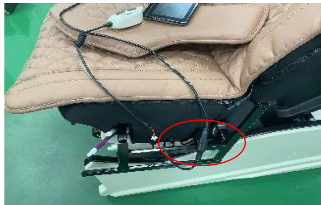
E. disconnected the terminal
