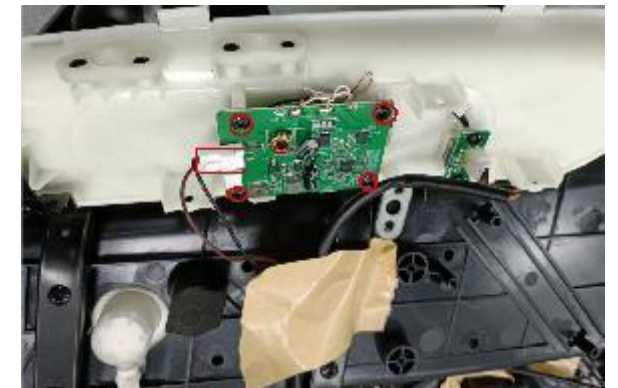
F. Disconnect the port and remove the 4 screws
