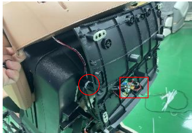
E.cut the cable tie, discontent 2 terminals
