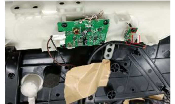
C. Disconnect the port and remove the 2 screws
