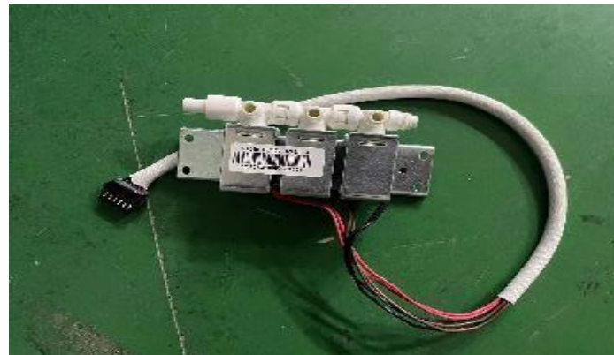
K.remove the 3-way air valve
