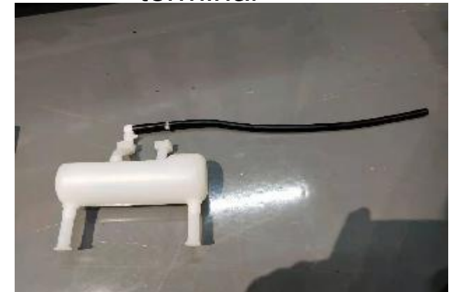
C. discontnet the air hose and terminal
