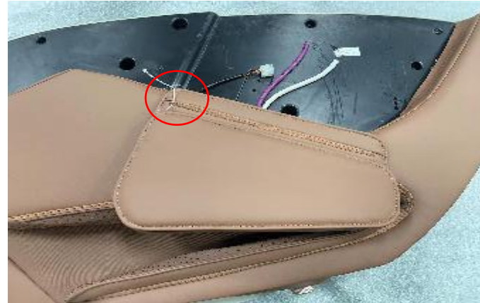
B. separate the leather from plastic screw
