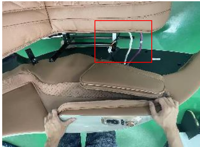
E. Disconnect the terminal and air hose
