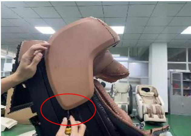
J .open the cover with a “—” screwdriver
