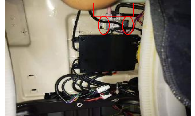
C.remove the screws, discontent the terminals, remove air valve
