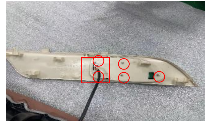
F. remove 5 screws, discontent the tterminal
