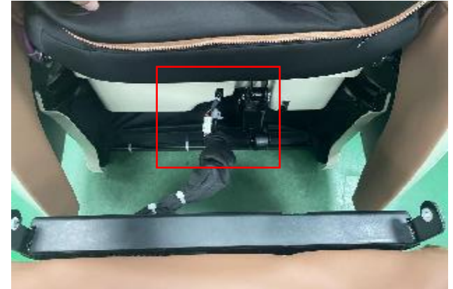
C.disconnect the terminal and air hose
