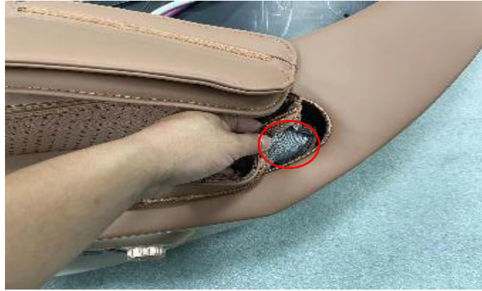
B. separate the leather from plastic screw
