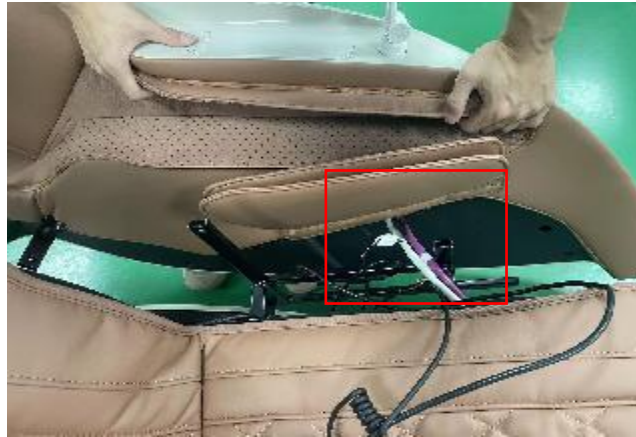
B. Disconnect the terminal and air hose
