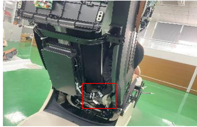
N .cut the cable tie, discontent the terminal
