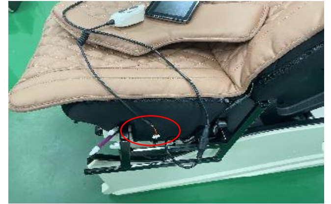
C. disconnected the terminal
