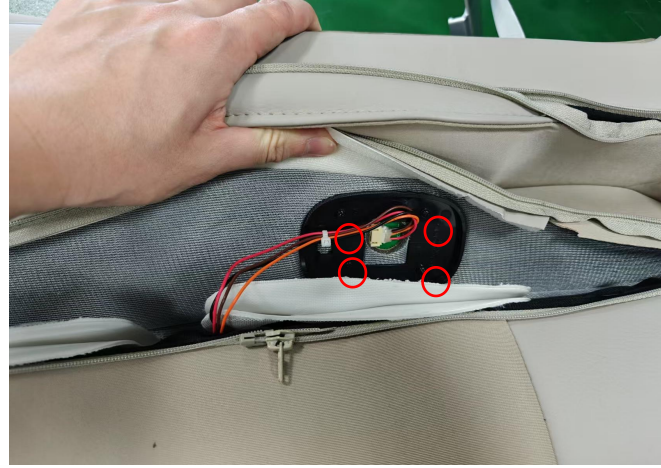
Remove 4 screws, cut off the zip ties, and unplug the terminals
