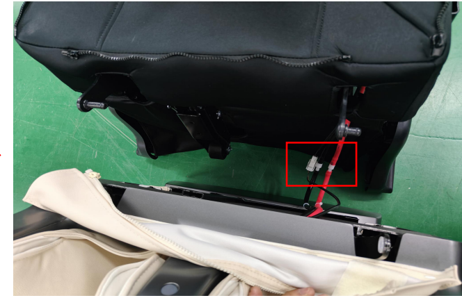
Remove the trachea and terminals
