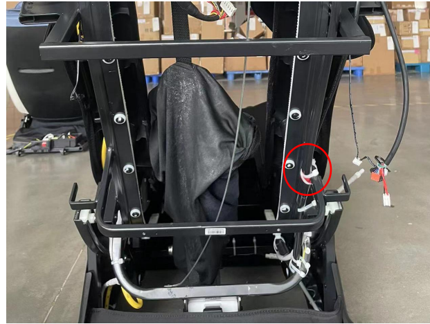
Cut off the backrest wire cable tie
