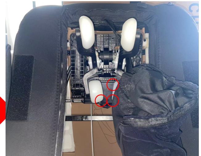
Remove the 3 screws on the upper cover of the movement adapter plate
