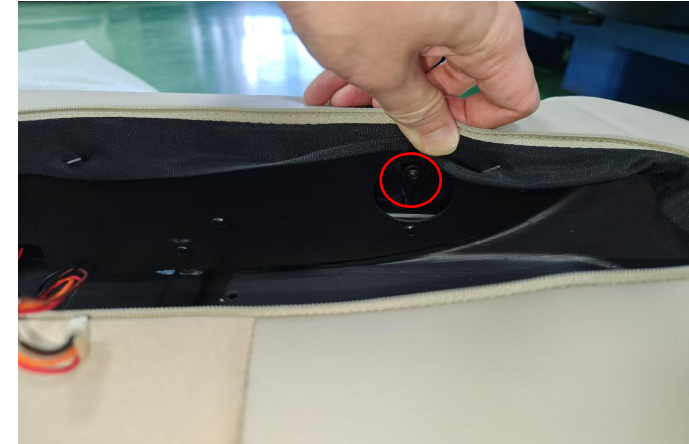
Remove the soreness detection handle
