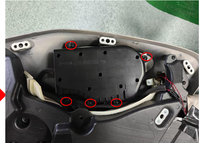
Remove the screws
