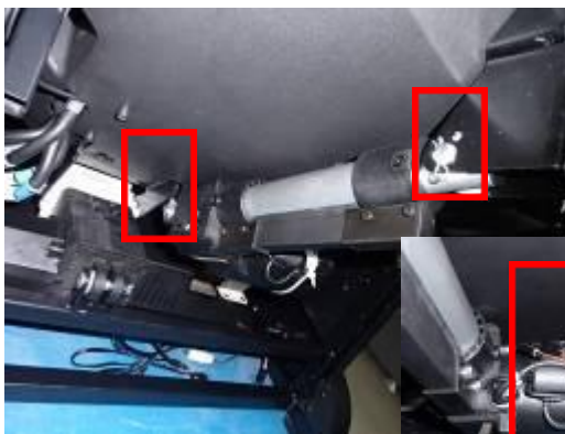
抬起小腿拆下前档板,之后定位图中三个位置,除下它们即可(建议先拆上方销轴以方便拆底部销轴) Pull-up the legrest and disassembly the plate washer then location map of three position, (moving the top of pin first)
