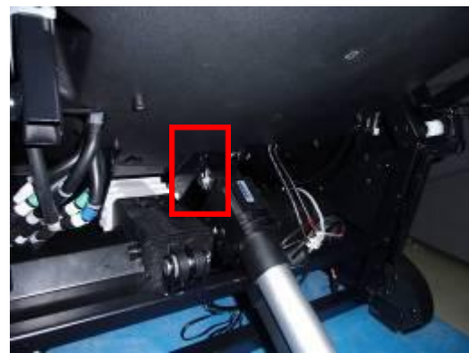
抬起小腿拆下前档板,之后定位图中三个位置,除下它们即可(建议先拆上方销轴以方便拆底部销轴) Pull-up the legrest and disassembly the plate washer then location map of three position, (moving the top of pin first)
