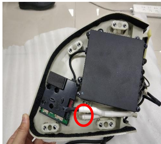
12. Unplug all the air hose to replace all the airbags
