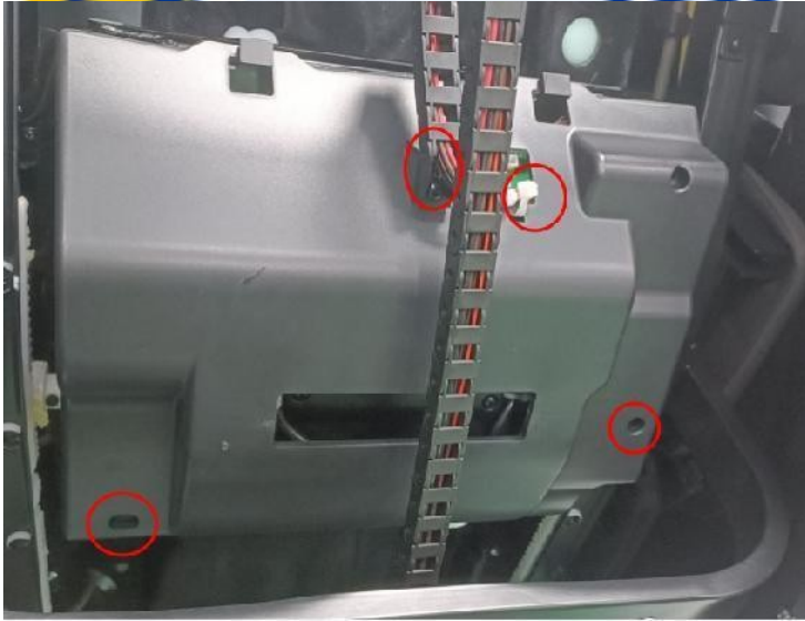
1.remove 4 screws and cut cable tie
