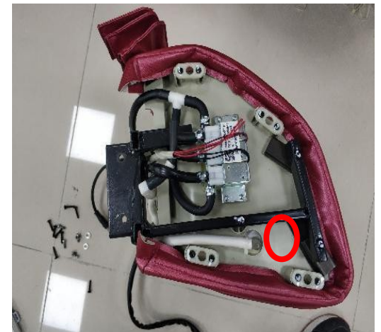
12. Unplug all the air hose to replace all the airbags
