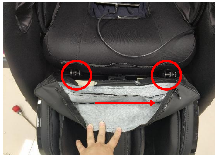
2.Remove the blocking on both sides of the legrest
