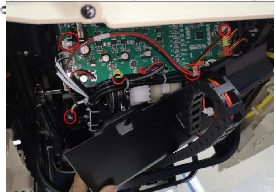
3 Unplug the terminal, remove the ground wire, and cut the cable tie
