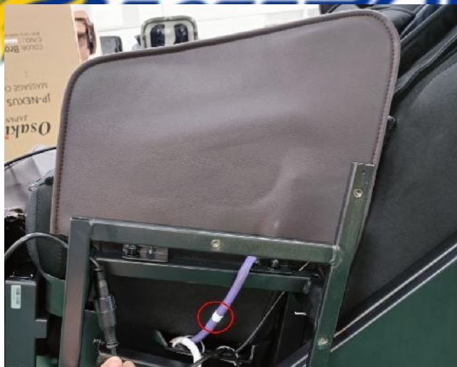
1 Disconnect the air hose interface
