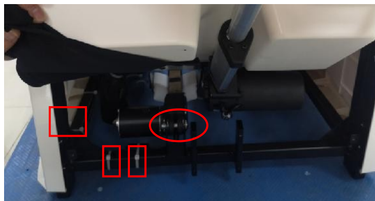
E.cut cable , remove the shaft
