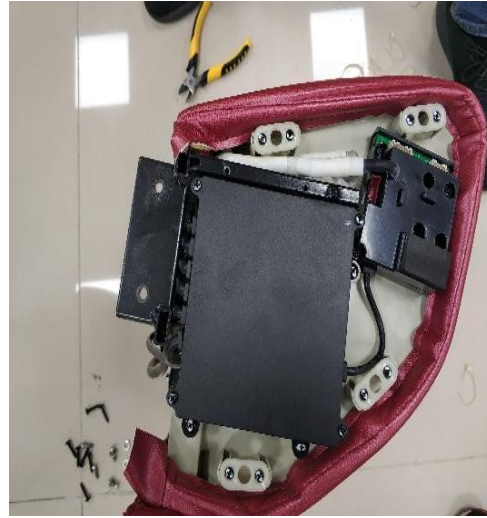
10. Tear off the sticky fur buckle to replace the upper legrest leather cover
