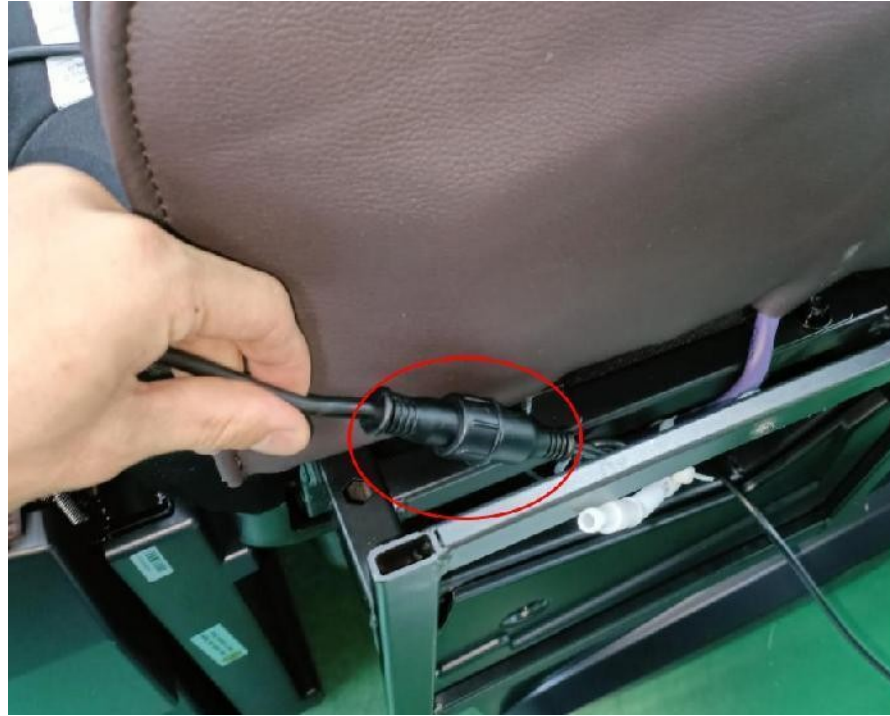
2 Disconnect the plug terminals
