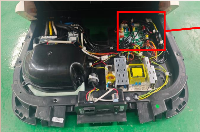
B.disconnect the terminals, remove 4 screws
