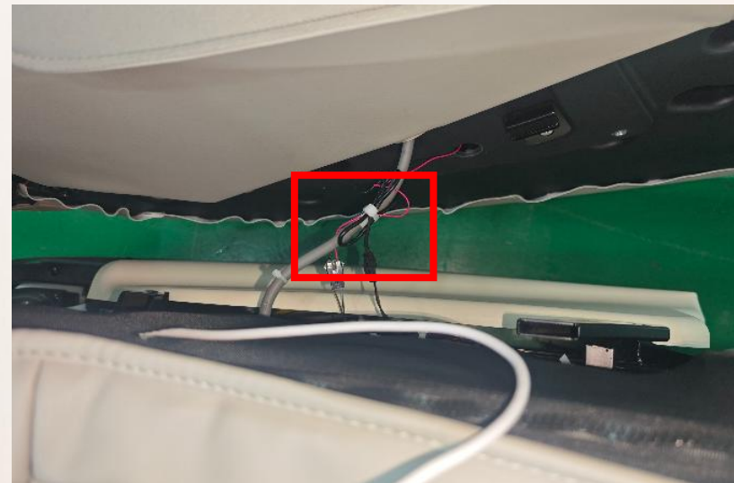
I.Cut off the tape clips
