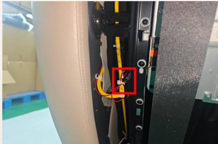
D.Cut off the tape clips
