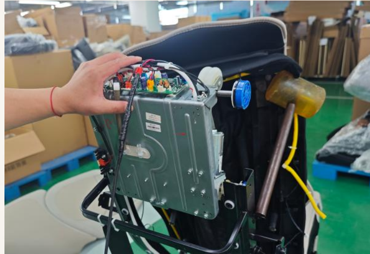
H.remove the gear box
