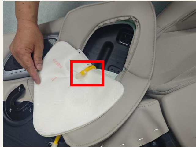
I. remove the air hose
