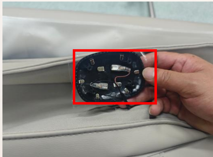
C.Disconnect the connection line
