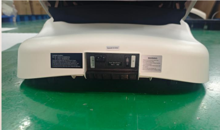
A.remove 2 screws, open themain PCB box
