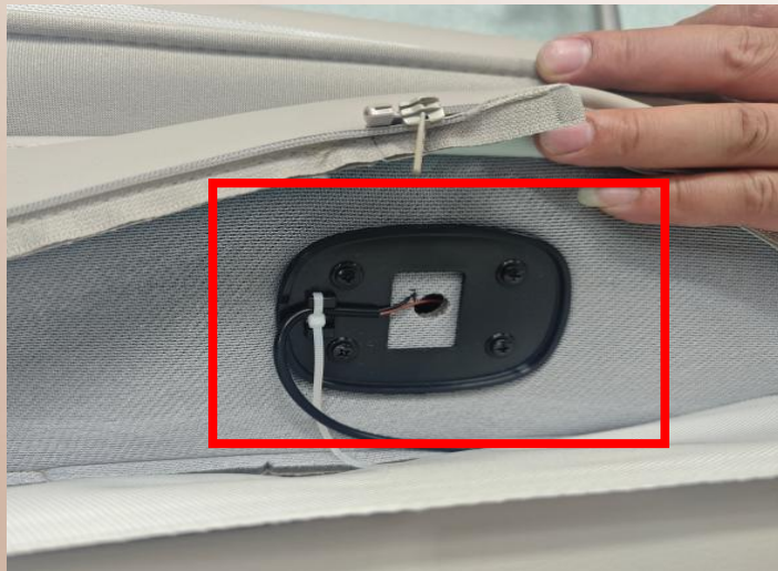
B. remove 4 screws
