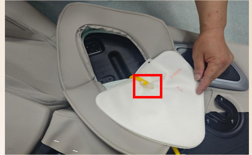
F.Cut off the tape clips
