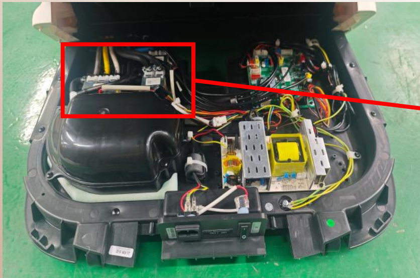
F. cut off the cable ties and remove the terminals.
