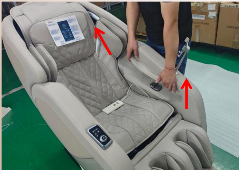
H.First, lift the side panel upwards, and then remove the side panel from the rear.
