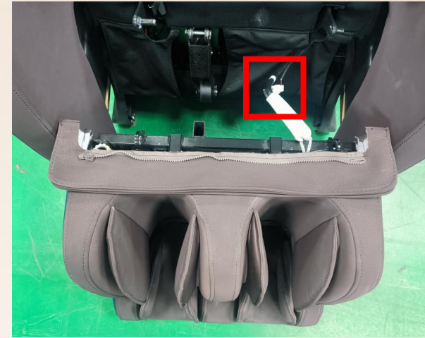
C.disconnect the air hose and wiring terminal
