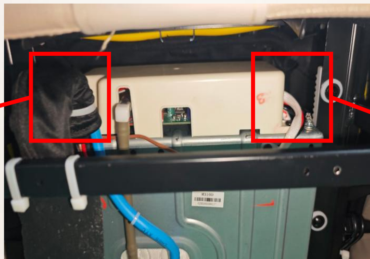
C.remove 5 screws ,remove the top cover
