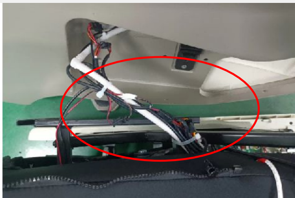
Cut off the buckle and disconnect the signal terminal
