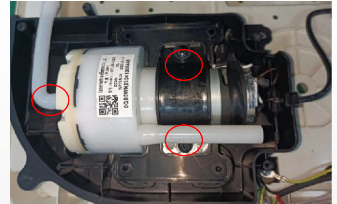
Remove 2 screws, Disconnect the air hose
