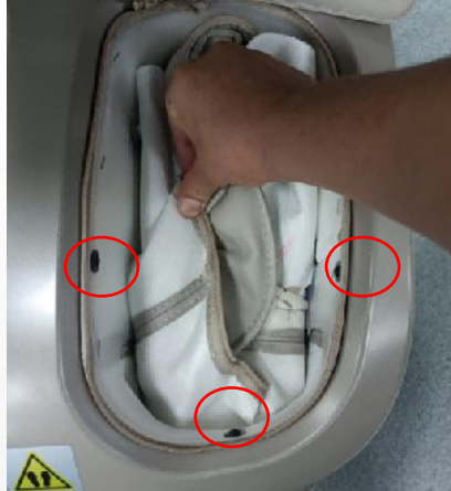
Remove 3 screws and pry out U-shaped nails
