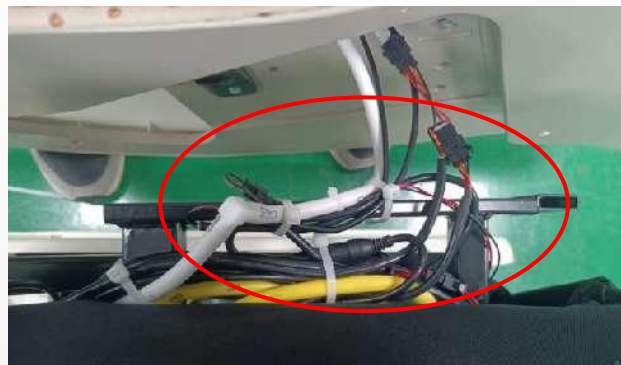
Cut off the buckle and disconnect the signal terminal
