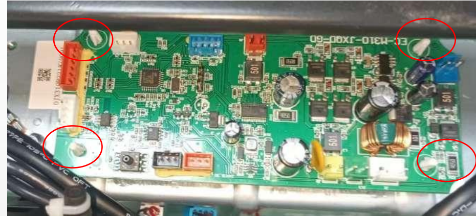
Remove the 4 Insulating column
