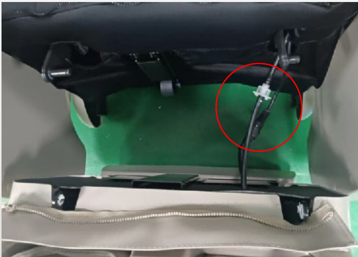
disconnect the air hose and terminals
