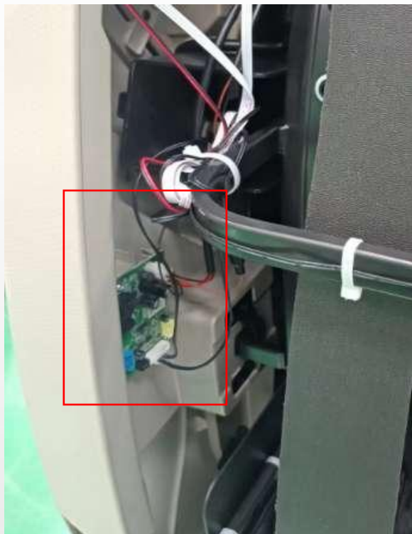
disconnect the signal terminal
