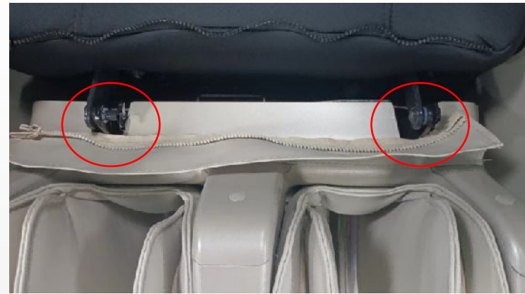
remove 2 limit baffles
