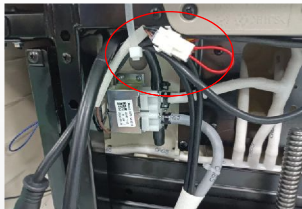
Cut off the buckle and disconnect the signal terminal
