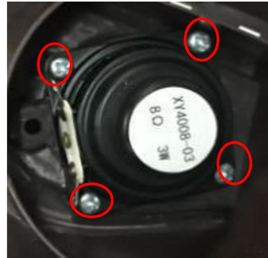
Remove four screws and replace the horn
