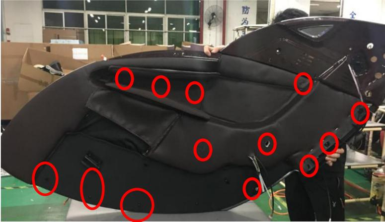
remove 15 screws separate the right side panel
