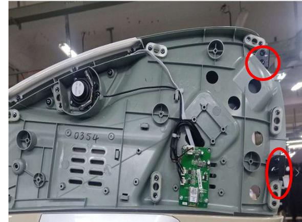
Remove the four screws on the left side of the hood
