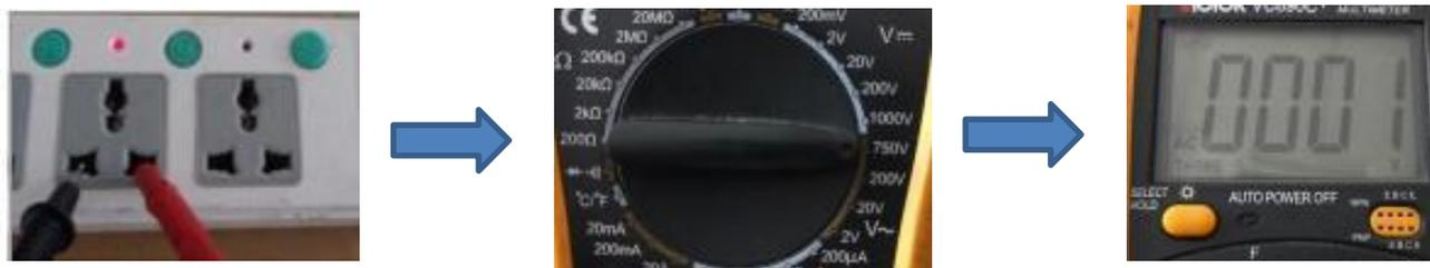
As shown in the above picture: measure the power supply (220V) of our household plug-in board, select the range of 750, and the test result is displayed as "001", indicating that the actual voltage of this group of sockets is 0V at the moment (the switch is not pressed down, so there is no power, and the light is not on).
