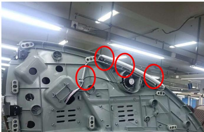
cut the cable tie, remove 3 screws
