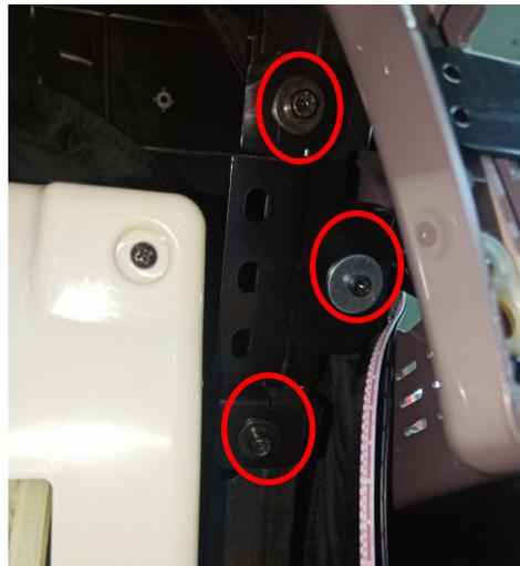
remove 6 screws, remove the iron
