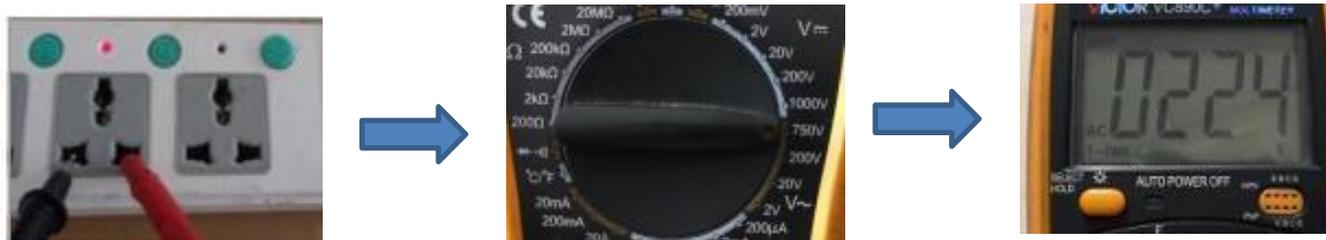
As shown in the picture above: measure the household plug-in board power supply (220V), select the range of 750, and the test result shows "224", indicating that the actual voltage of this group of sockets is 224v at the moment (the switch is pressed down, so there is power, and the light is on).
