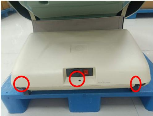
remove 3 screws, remove the cover
