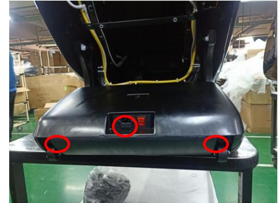
remove 3 screws fixing main PCB box
