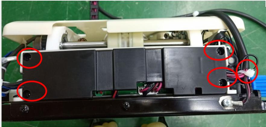
remove 4 screws, cut the cable tie
