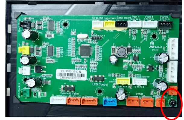
remove the screw and remove main PCB
