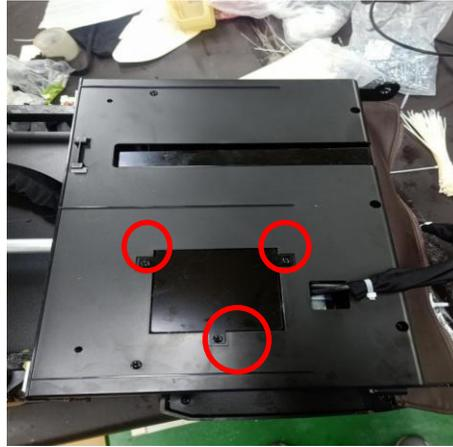
remove 3 screws fixing the box
