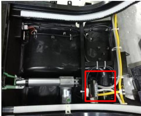
remove 2 screws and disconnect the terminal
