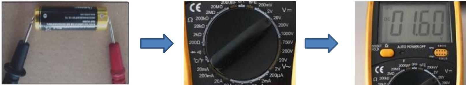
As shown in the picture above: the test result is "1.58", indicating that the voltage at both ends of the battery is 1.58v, and the red lead is connected to the "+" pole of the battery, and the black lead is connected to the "-" pole of the electromagnetic.
