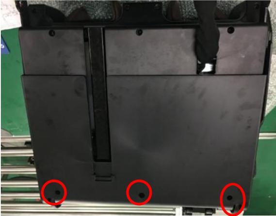
remove 3 screws fixing the rear cover
