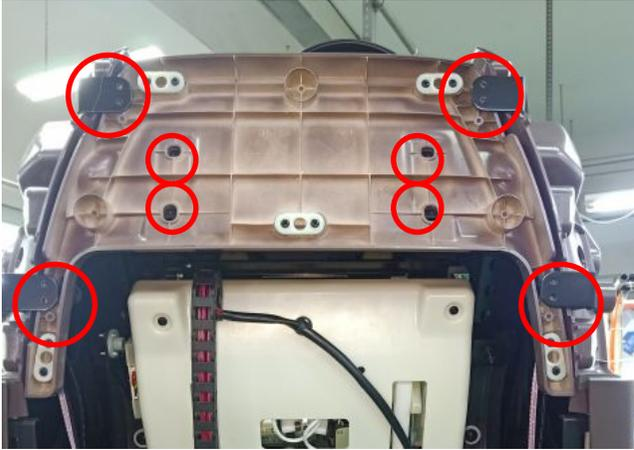
Remove 8 screws with cross screwdriver
