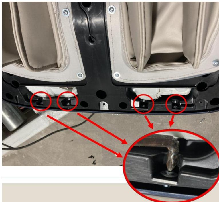
17: devided all the air pipe connector as photo below;
