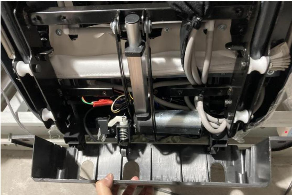
5: As photo below, remove the R- shaped bolt in the joint;
