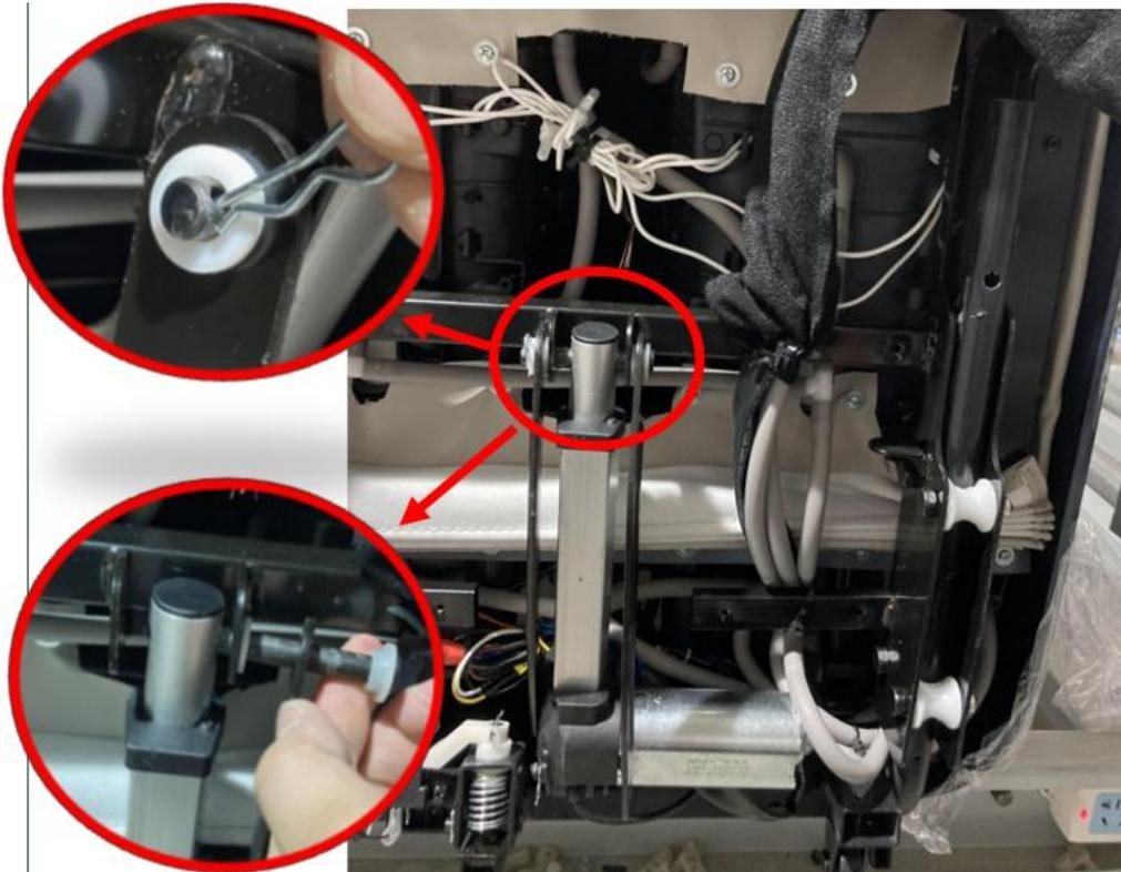
6: As photo below, turn over the pushrod, remove the R- shaped bolt in the joint again and cut the plastic fixture.
