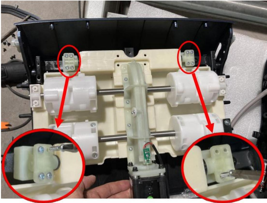
22: As photo below, divided the cable of the foot roller moter.
