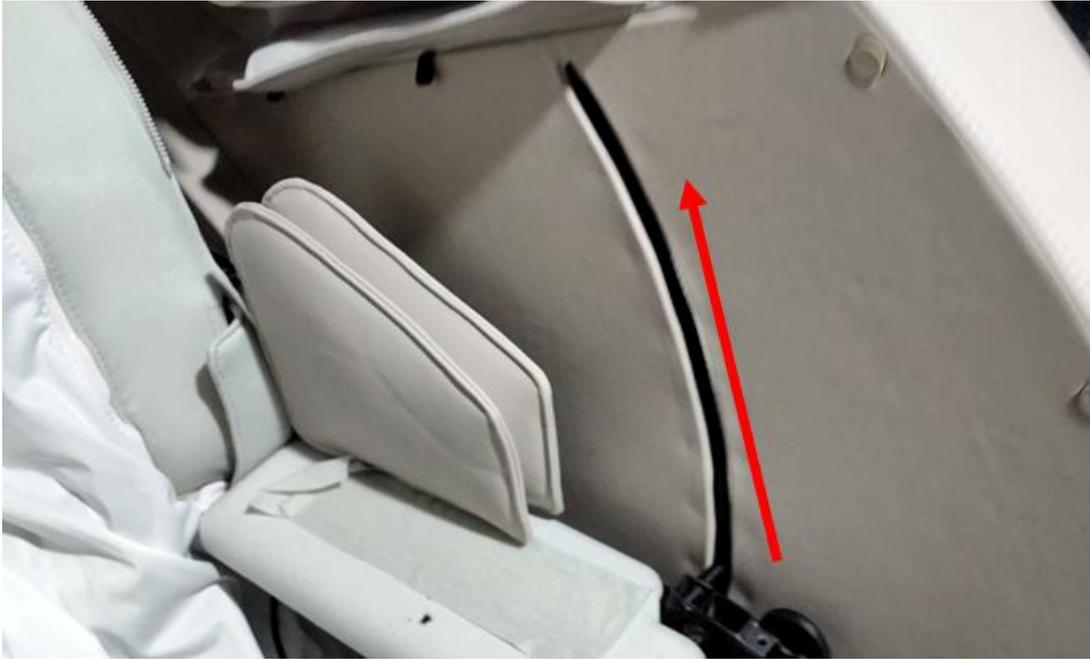
4: As photo below, after lifting the panel to the limit, pull the whole panel out lightly.
