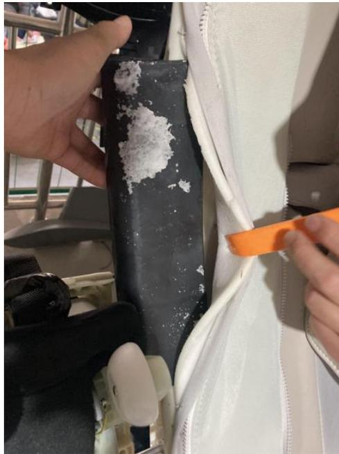
3: As photo below, without black plastic position limiting component, mechanism can be removed accordingly.
