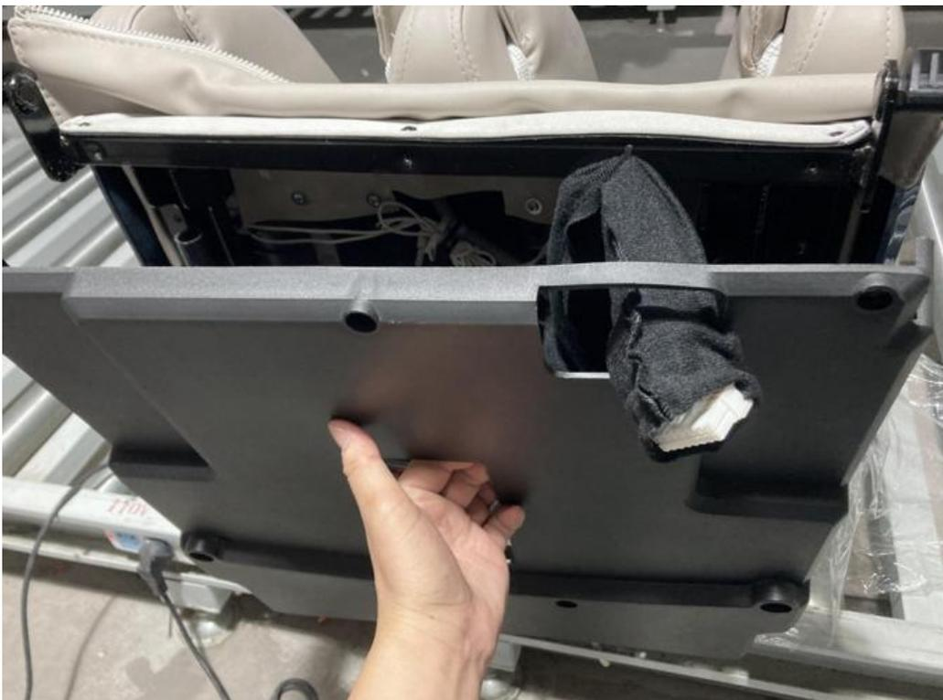
3: As photo below, remove the two screws on both side;
