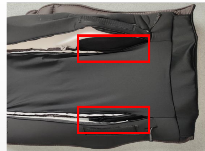
H.Tear open the adhesive button to remove the heating wire
