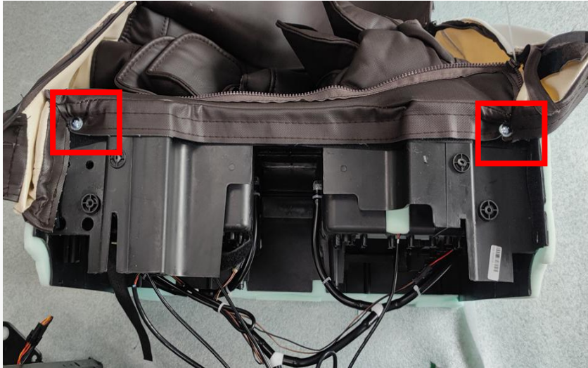
Q. remove 4 screws ,tear open the sticky button
