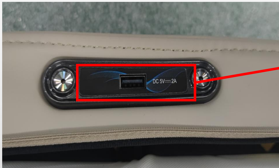
K.tear open the veneer,remove 2 screws
