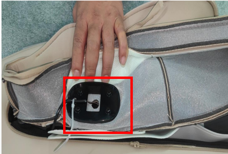
G.cut off the zip ties,remove 4 screws
