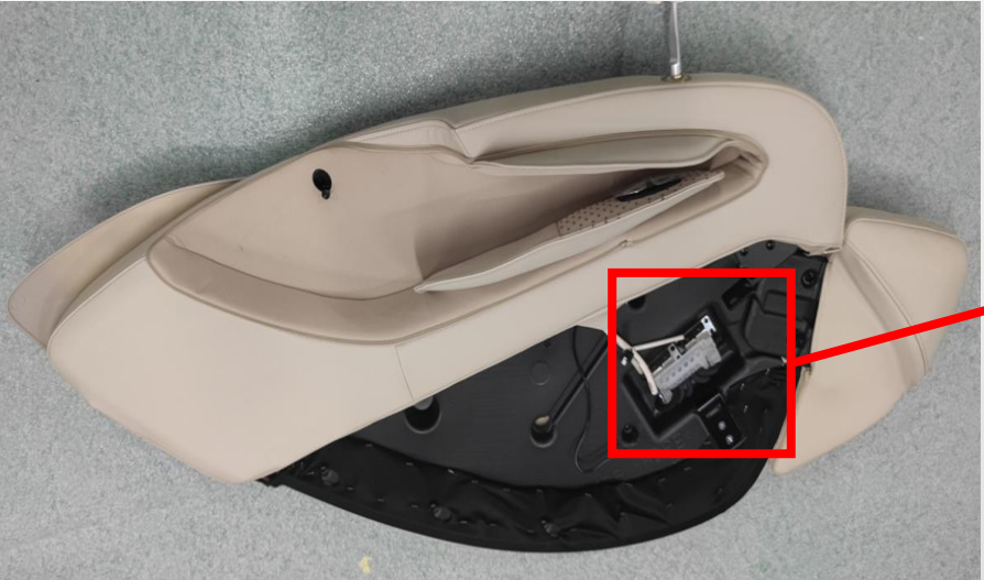
B.remove 8 screws,remove the trachea
