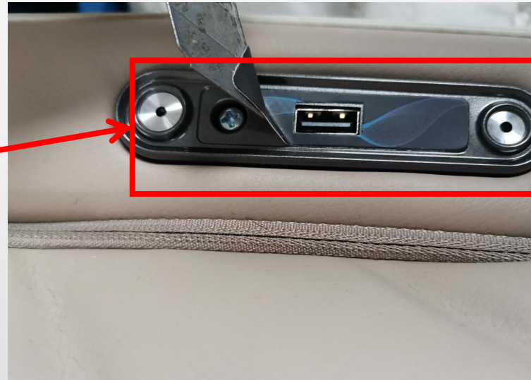
K.tear open the veneer,remove 2 screws
