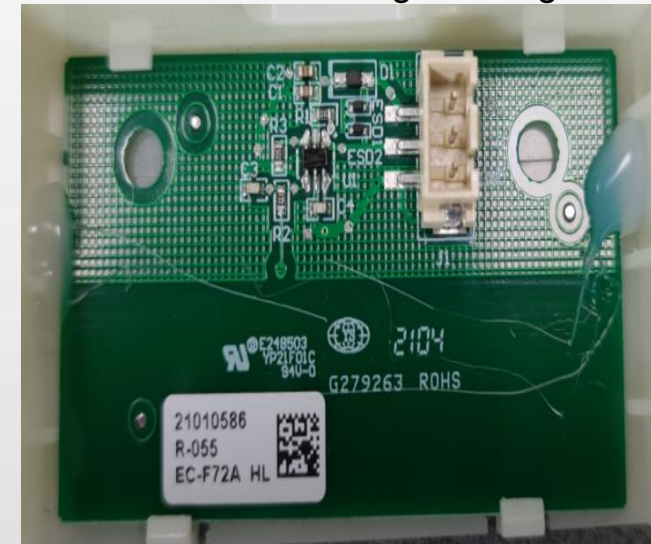
Leg length detection PCB
