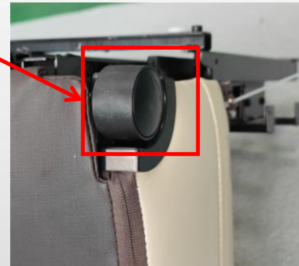
G. remove the covers on both sides of the casters and remove the 4 fixed screws
