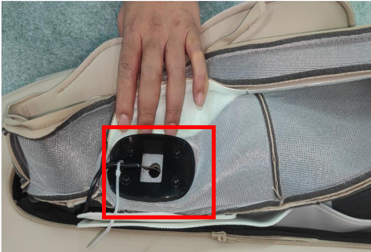
E.cut off the zip ties,remove 4 screws
