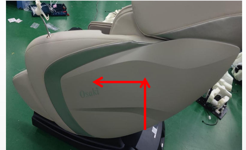
B.Lift up the front end of the side panel and then move the entire side panel forward
