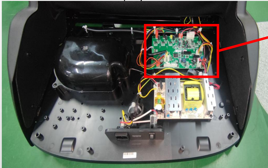
B.disconnect the terminals, remove 4 screws
