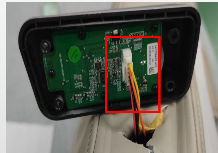
P.disconnect the connecting wire
