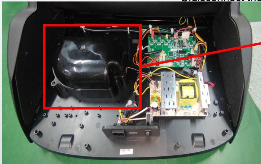
C.disconnect the terminals, remove 4 screws
