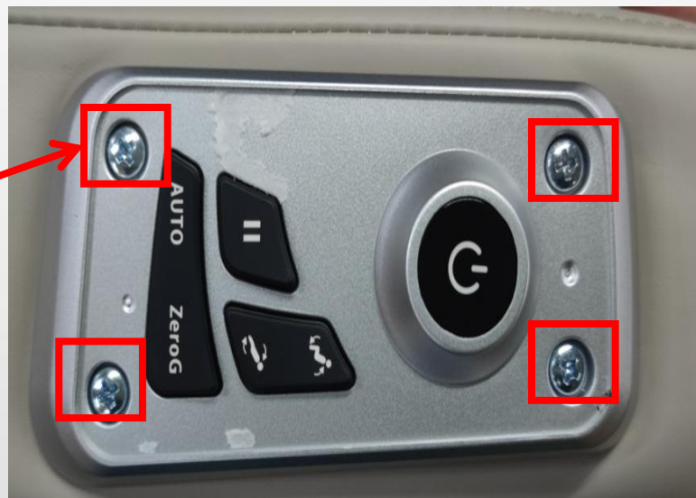
O.tear open the veneer,remove 2 screws
