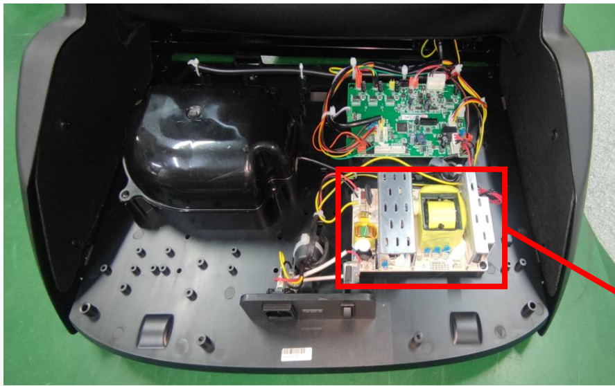
C.disconnect the terminals, remove 4 screws
