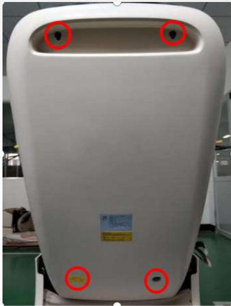
1. 拆卸4颗螺丝取下后盖 Remove the four screws to take off the back cover.
