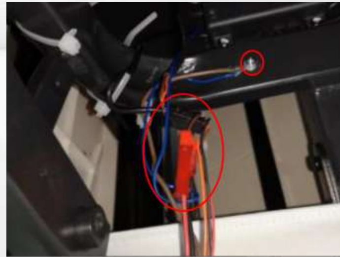
8.断开端子并拆卸1颗地线螺丝 Disconnect the terminal and remove one ground screw.
