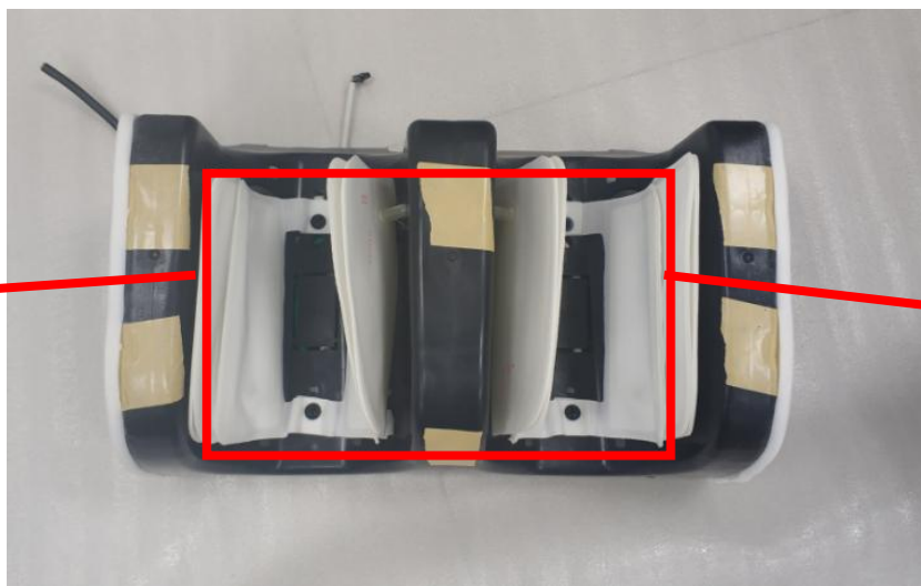
remove the screws fixing air bag page 40
