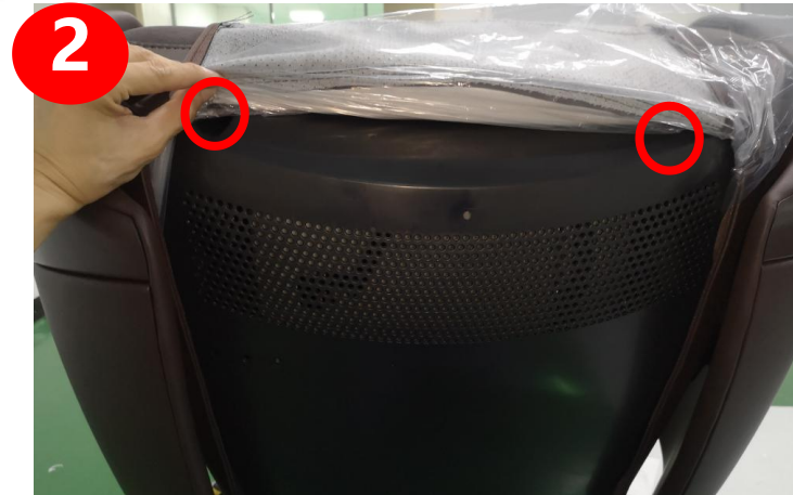
remove 2 screws on the top
