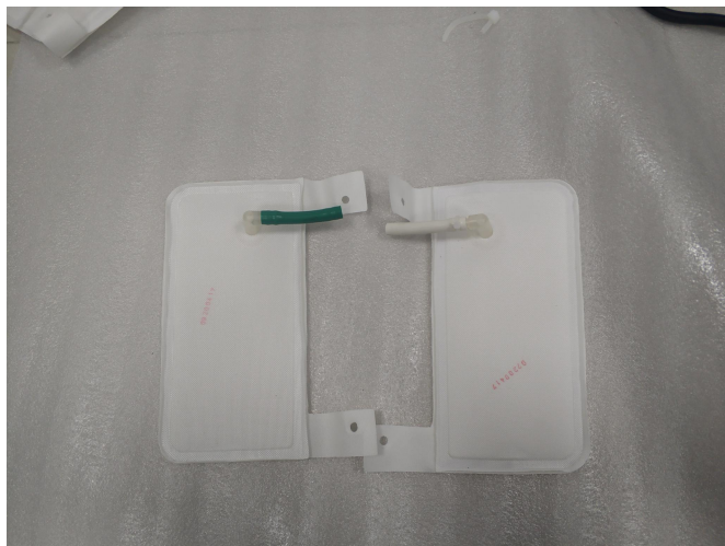
cut cable tie, disconnected the air hose
