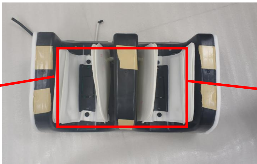
remove the screws fixing the air bag
