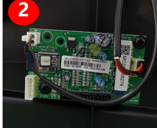
disconnected the terminals and remove 4 screws
