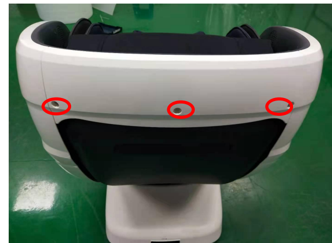
Remove 2 screws from left and right shoulder
