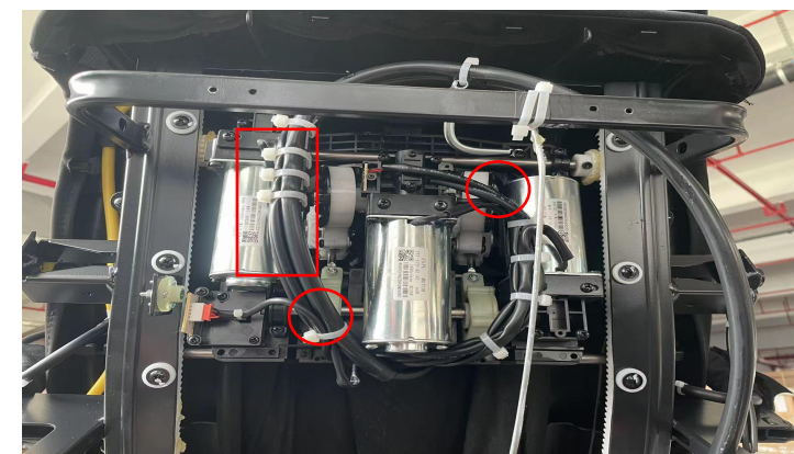
cut the cable ties remove 4 screws
