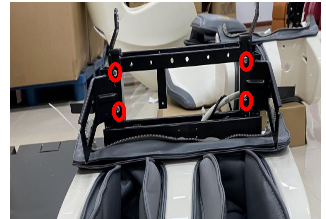
Remove the 4 screws and hardware
