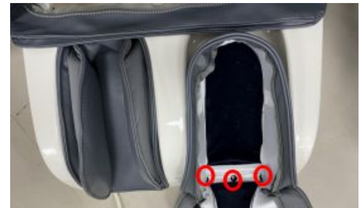
Remove the 3 screws and remove the holster
