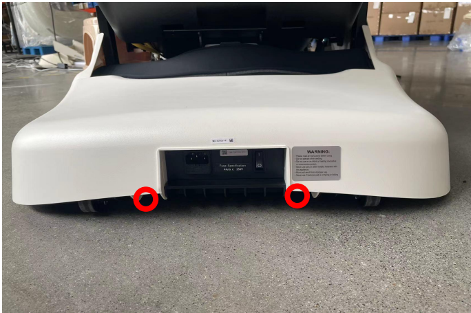
Remove the 2 screws and remove the top cover of the center box
