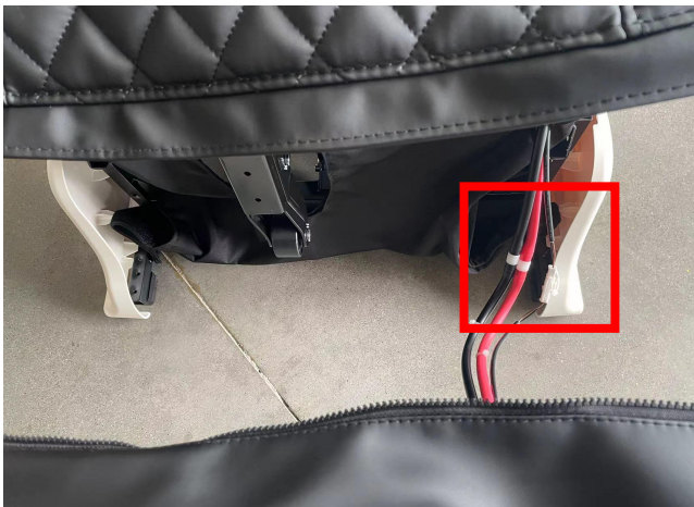
Disconnect the terminal and air pipe
