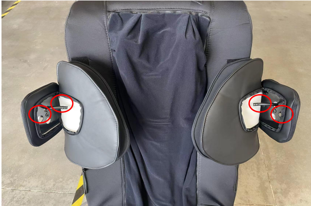
Remove 2 screws and disconnect the air pipe
