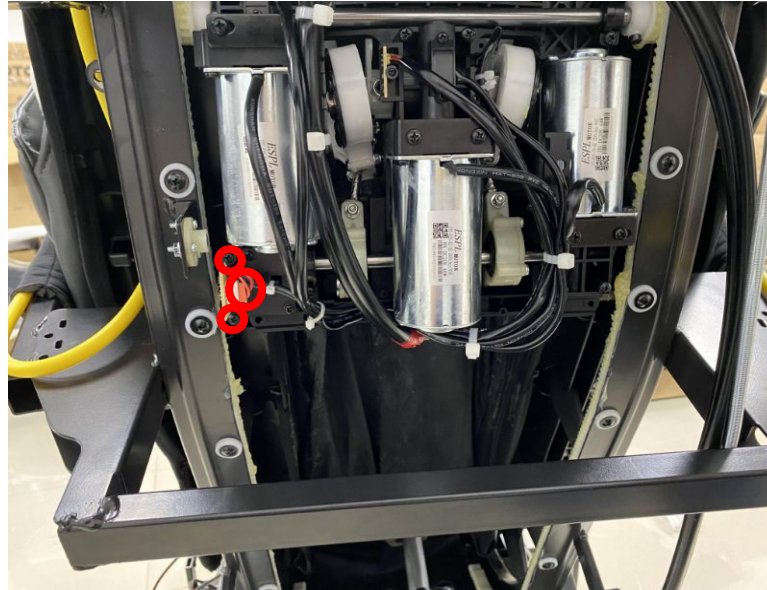
Remove 2 screw disconnect terminals
