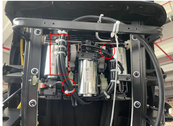
cut the cable ties and remove 4 screws
