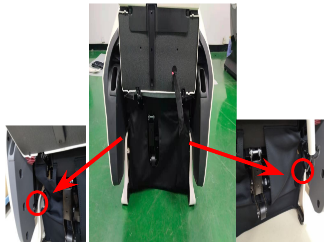
Lift calf and remove 2 screws
