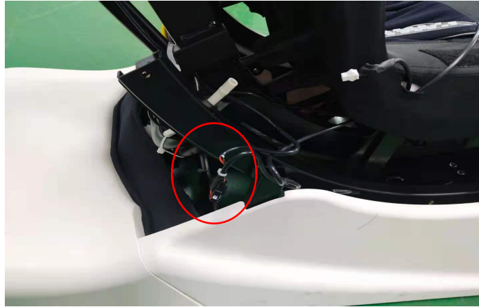
cut the cable ties and disconnect the terminals
