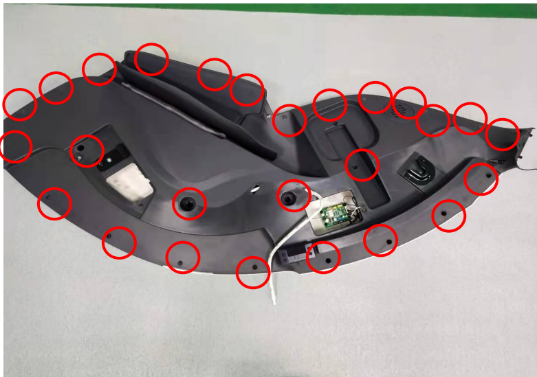
Remove the 13 plugs and 27 screws, and remove the outer cover of the side panel
