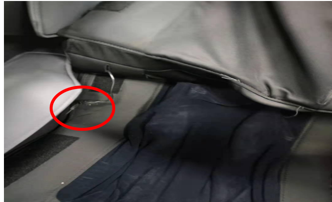
Cut the tie disconnect terminal
