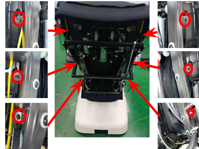
Remove 6 screws on backrest
