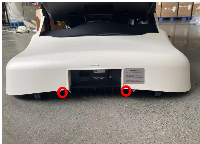
Remove 2 screws and remove center box cover
