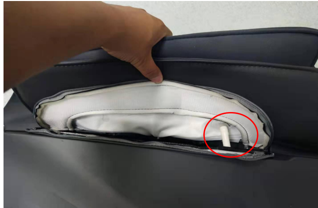
Remove the air bag and cut the tie to disconnect the trachea
