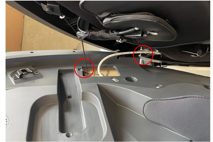
Disconnect the terminal and air pipe
