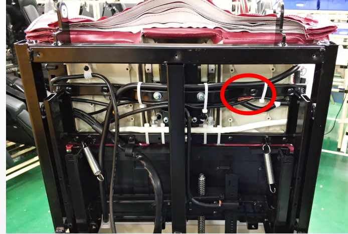
cut cable tie, disconten the terminal
