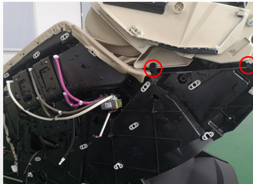
remove 2 screw, then remove left side panel
