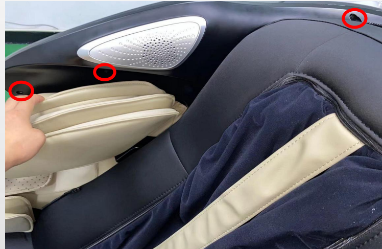
remove 3 screws and remove the hood cover
