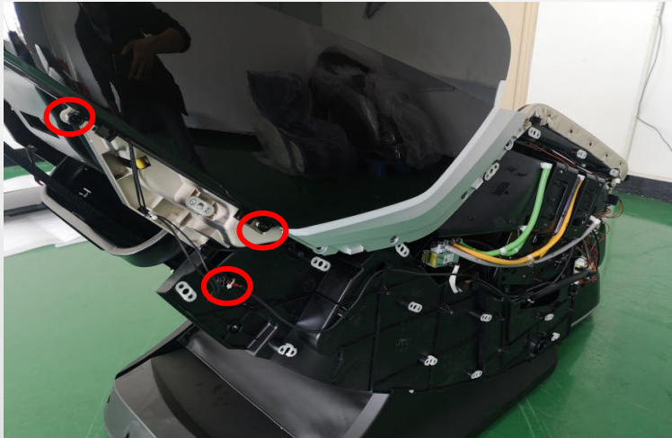
remove 2 screws and discontent the terminal
