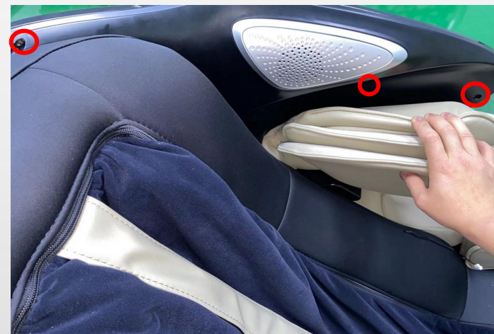
remove 3 screws and remove hood cover
