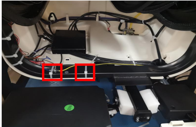
cut the cable tie
