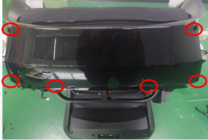
remove 6 screws and remove the cover
