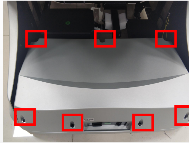
remove 7 screws and remove the cover
