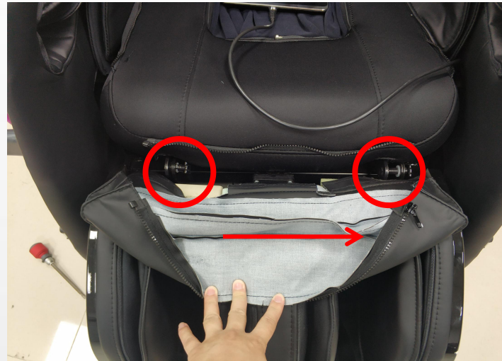
remove 2 baffle, move out legrest towards the right
