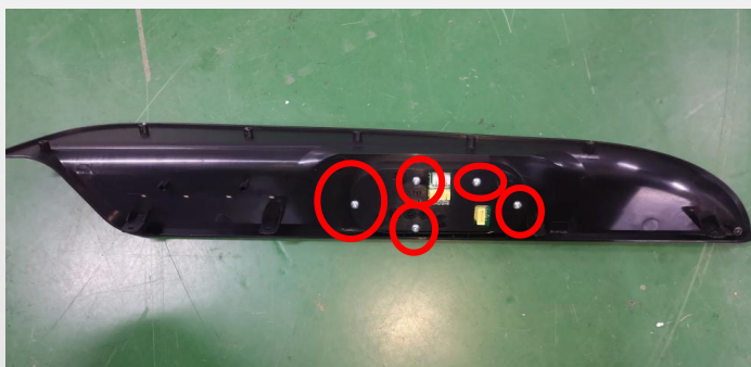
remove 5 screws, remove the control
