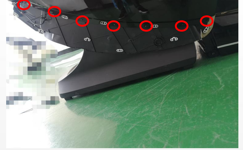
remove 7 screws and remove upper cover
