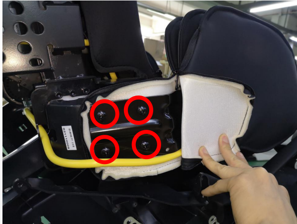
remove 4 screws and remove the shoulder
