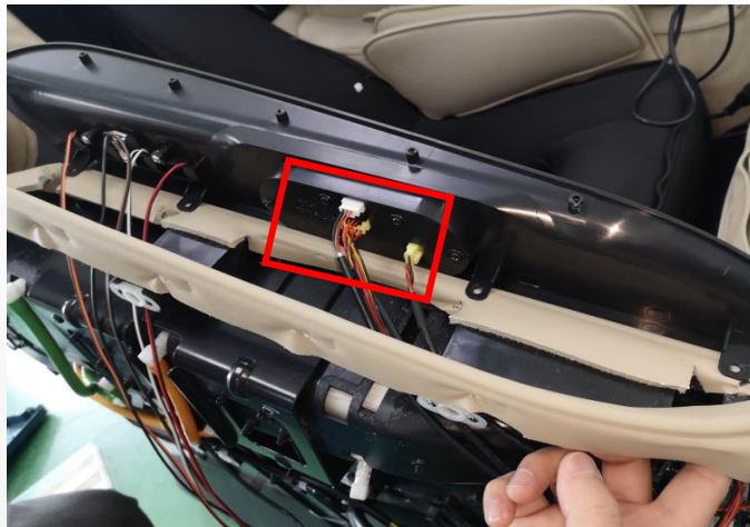
discontent the terminal and remove the cover
