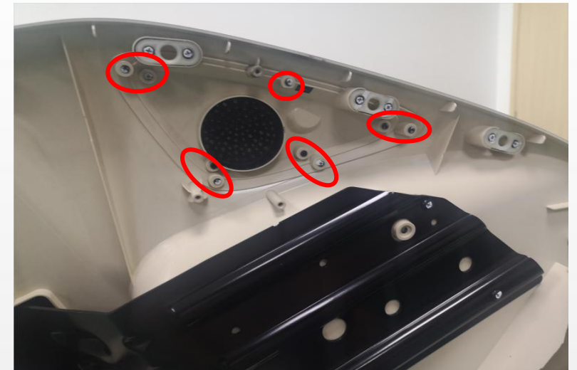
remove 9 screws, remove the horn net cover
