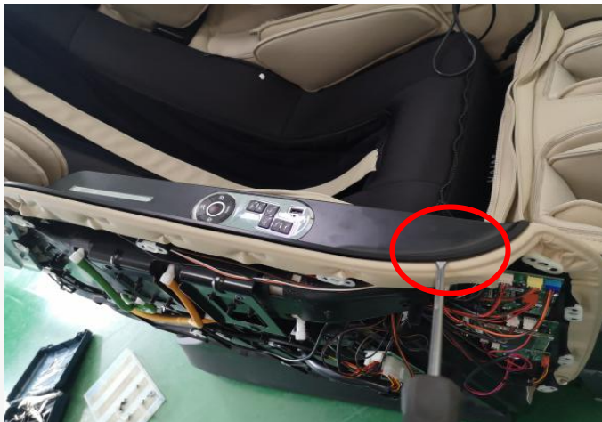
open the cover with a “—” screwdriver
